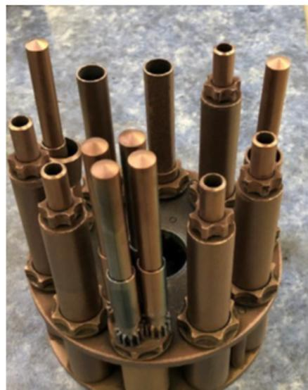
**Figure 5.** Method of samples' location in stainless-steel housing.
