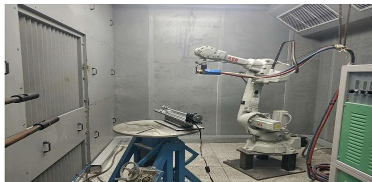
**Figure 1.** Atmospheric plasma-spraying equipment.
