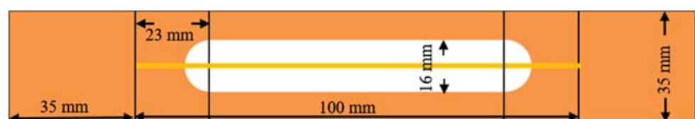
Figure 4. Schematic diagram of fiber monofilament tensile processing and molding sample.
