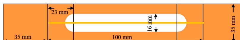
**Figure 4.** Schematic diagram of fiber monofilament tensile processing and molding sample.
