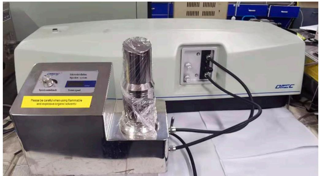
Figure 1. Laser particle size analyzer.
