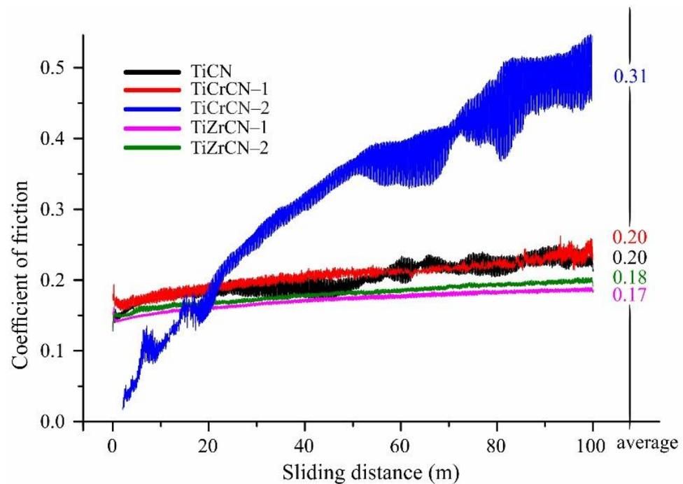
**Figure 6.** CoF with an average value for TiCN, TiCrCN, and TiZrCN coatings on a titanium VT1-0 substrate.
