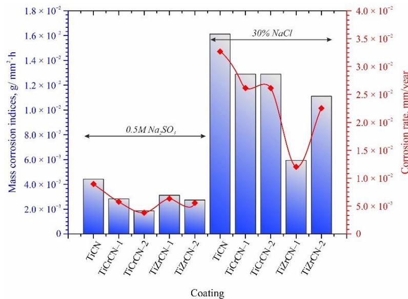
**Figure 9.** Corrosion indices of TiCN, TiCrCN, and TiZrCN coatings on a substrate of titanium VT1-0.
