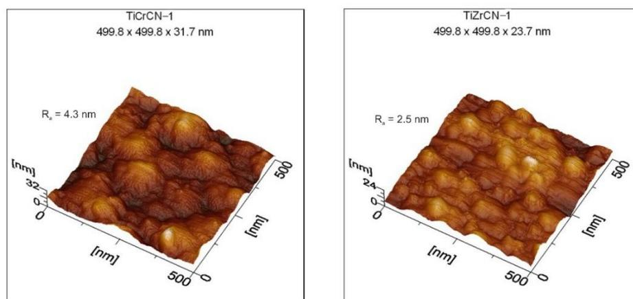
**Figure 4.** SPM images of the topography of deposited TiCrCN-1 and TiZrCN-1 coatings on titanium VT1-0.
