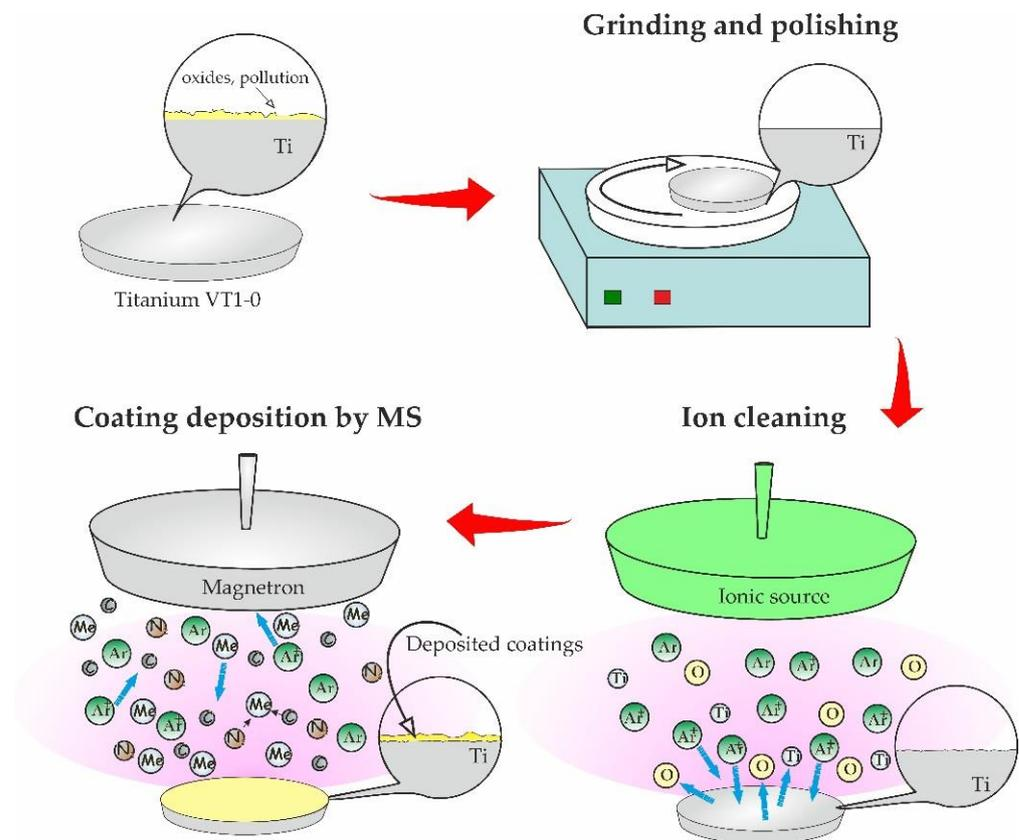
**Figure 2.** Scheme of the process of preparing the substrate and coating deposition.
