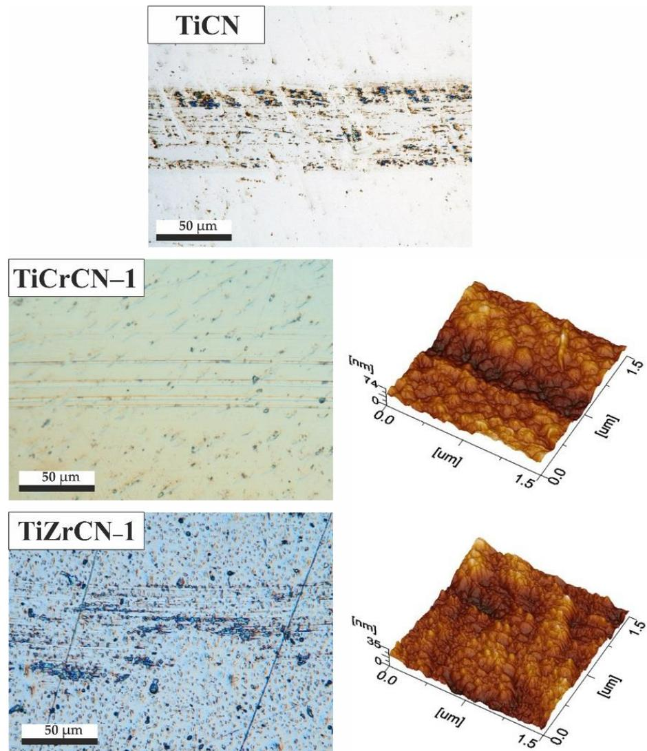
**Figure 7.** Optical micrograph and SPM images of the wear track of coatings after tribological tests.
