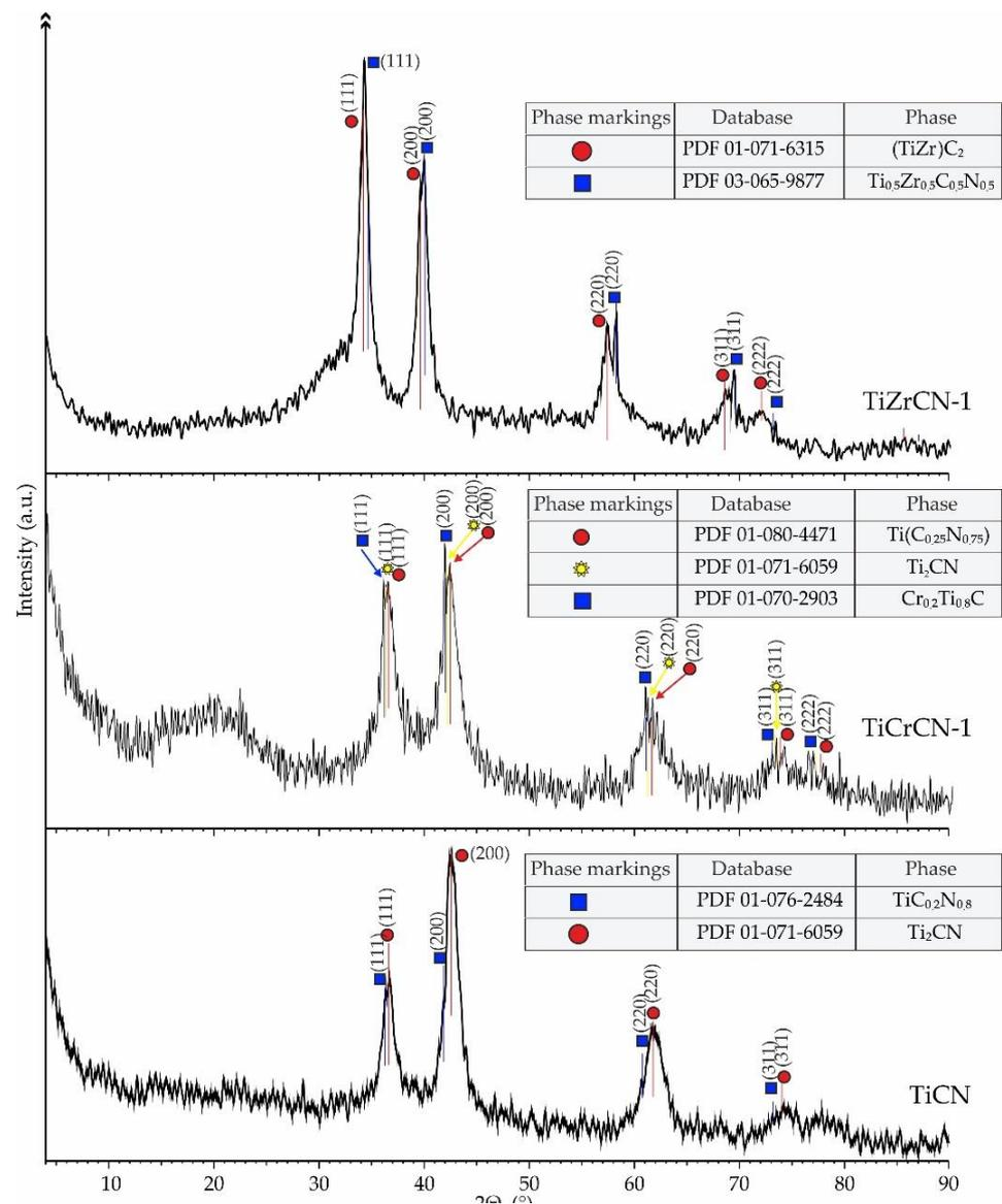
Figure 5. XRD patterns obtained for TiCN, TiCrCN-1, and TiZrCN-1 coatings.
