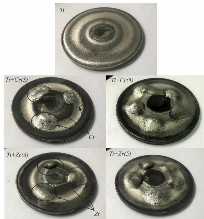
**Figure 1.** Titanium and composite targets after deposition of TiCN, TiCrCN, and TiZrCN coatings.
