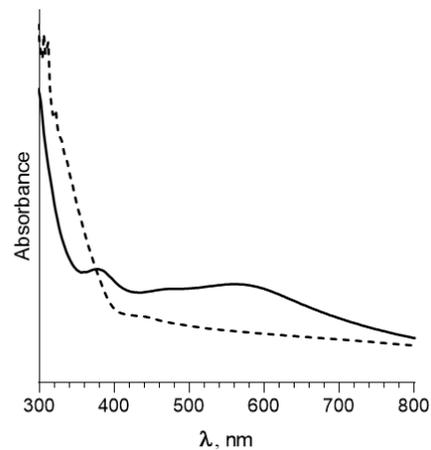
**Figure 2.** The optical spectra of AgCl sample before (dashed line) and after (solid curve) sunlight irradiation.
