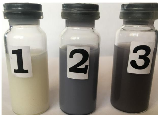
**Figure 1.** Colors of silver chloride sol in a solution simulating sweat after 7 days of storage: sample 1—in a dark place, sample 2—in diffused sunlight, and sample 3—in direct sunlight.
