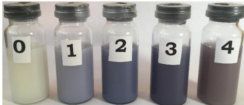
**Figure 4.** Samples of silver chloride sol. The photo was taken after three days of storage under different conditions. The concentration and storage conditions are shown in the second column of the Table 1.
