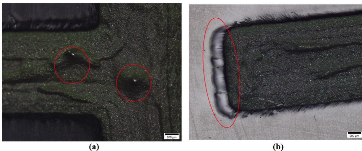
**Figure 9.** Characterization using optical microscope: (a) valley and mountain formation; (b) shadow electrodes.
