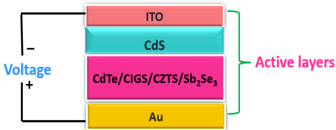
Figure 1. Schematic of various absorber layer-based solar cell.
