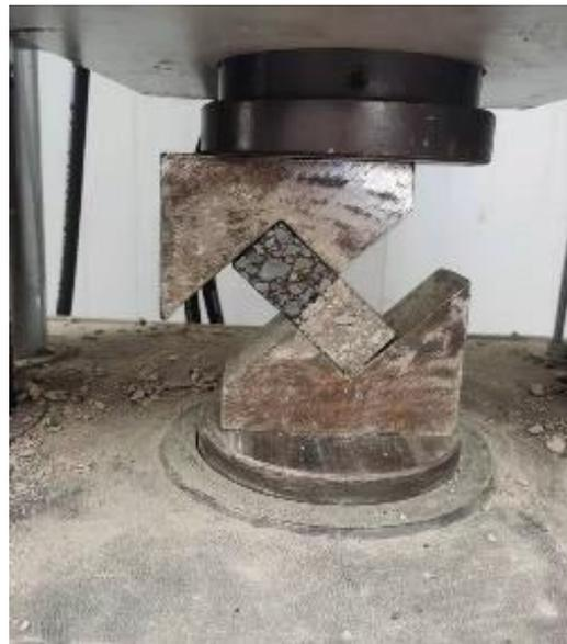
**Figure 2.** Inclined shear test device.
