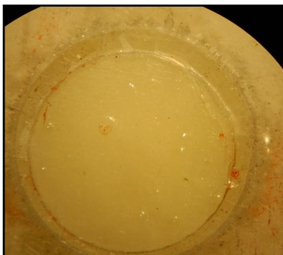
**Figure 7.** The specimen shows an adhesive type of bond failure.
