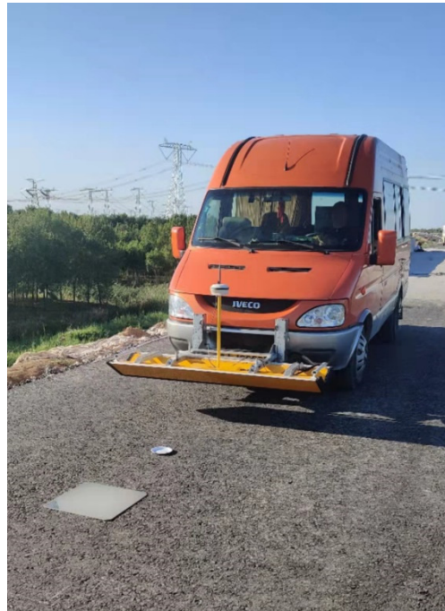
Figure 1. Three-dimensional ground-penetrating radar (GPR) inspection vehicle.
