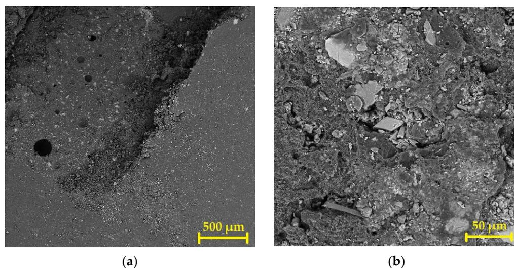
**Figure 12.** SEM photomicrographs of the coating with rounded particles (NBR-REF): (a) reference coating not exposed to the aggressive environment—50× magnification; (b) NBR-REF after exposure to CH<sub>2</sub>O<sub>2</sub> for 120 days—500× magnification.
