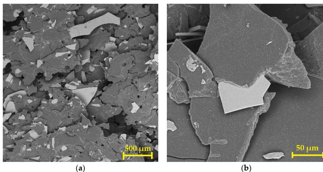
**Figure 13.** SEM photomicrographs of the coating containing glass flakes (NBR-GF): (a) reference coating not exposed to the aggressive environment—50× magnification; (b) NBR-GF after exposure to CH<sub>2</sub>O<sub>2</sub> for 120 days—500× magnification.
