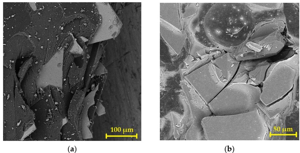
**Figure 16.** SEM photomicrographs of the coating NBR-GF containing glass flakes: (a) sample not exposed to the aggressive environment—300 $\times$  magnification; (b) sample after exposure to 30%  $\text{CH}_2\text{O}_2$  for 90 days—500 $\times$  magnification.
