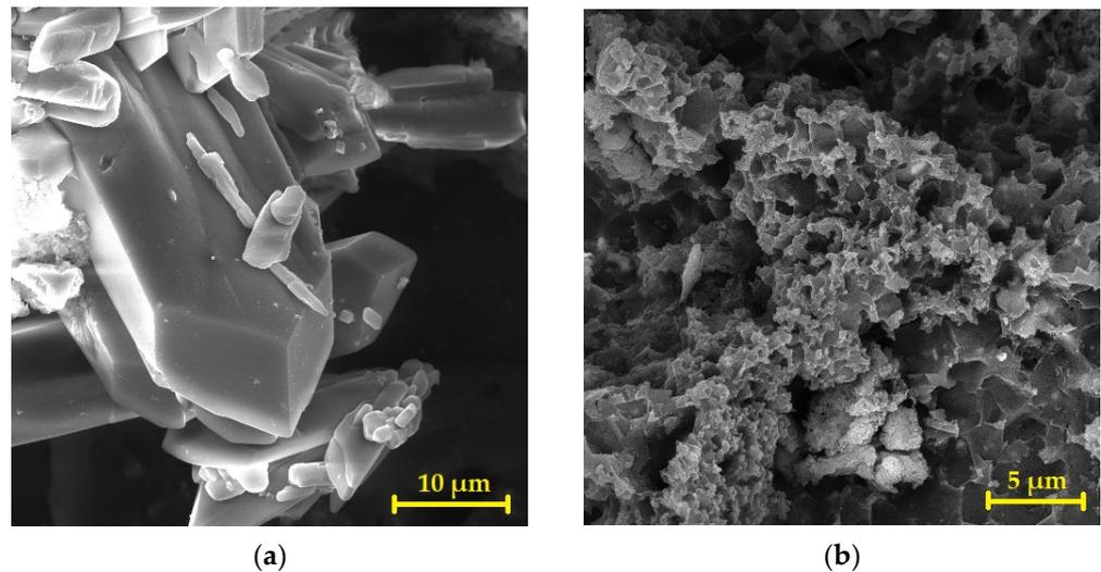
**Figure 15.** SEM photomicrographs of the coating after exposure to 30%  $\text{CH}_2\text{O}_2$  for 120 days: (a) NBR-CW containing shards exposed to the aggressive environment—3000 $\times$  magnification; (b) NBR-REF with rounded particles—5000 $\times$  magnification.
