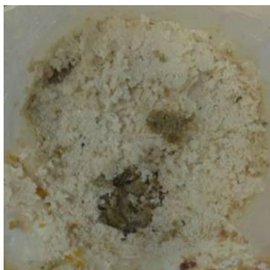
**Figure 9.** Complete degradation of the NBR-GF coating exposed to 30% CH<sub>2</sub>O<sub>2</sub> for 120 days.
