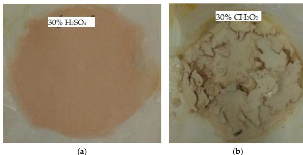
**Figure 8.** Coating NBR-GF after chemical stress: (a) colour change of the coating exposed to 30% H<sub>2</sub>SO<sub>4</sub> for 120 days; (b) cracking of the coating exposed to 30% CH<sub>2</sub>O<sub>2</sub> for 90 days.
