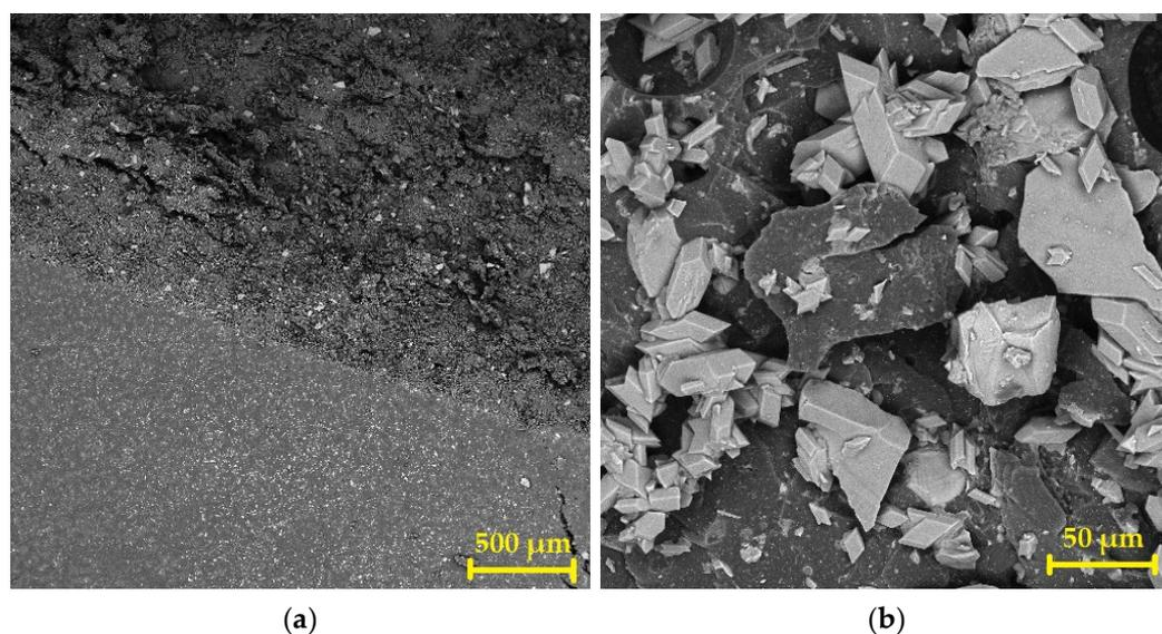
**Figure 14.** SEM photomicrographs of the coating NBR-CW containing shards from a windshield: (a) reference coating not exposed to the aggressive environment—50 $\times$  magnification; (b) NBR-CW after exposure to  $\text{CH}_2\text{O}_2$  for 120 days—500 $\times$  magnification.
