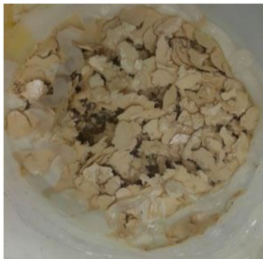
**Figure 7.** An example of complete degradation of the NBR coating with a filler of rounded particles (NBR-REF) exposed to 30%  $\text{CH}_2\text{O}_2$  for 120 days.
