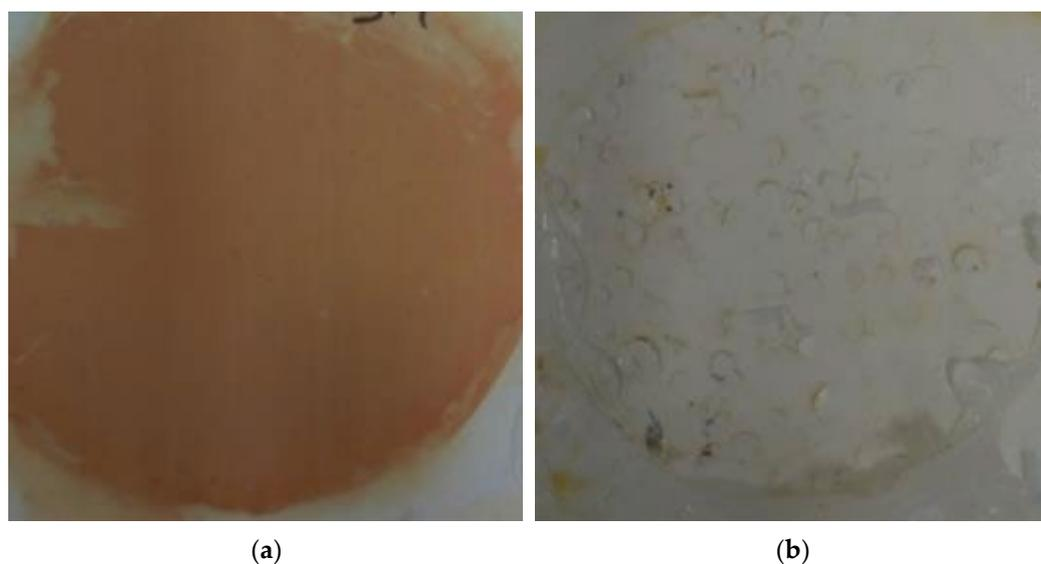
**Figure 6.** NBR-REF coating containing rounded silica particles after chemical loading: (a) colour change of the coating exposed to 30% HCl for 90 days; (b) cracking of the coating exposed to 30% CH<sub>2</sub>O<sub>2</sub> for 60 days.
