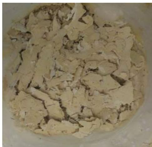
**Figure 11.** Complete degradation of the NBR-CW coating exposed to 30% CH<sub>2</sub>O<sub>2</sub> for 120 days.
