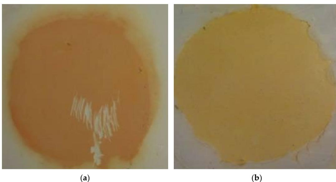
**Figure 10.** The NBR-CW coating: (a) colour change after 90-day exposure to 30% HCl; (b) colour change after exposure to 5% CH<sub>2</sub>O<sub>2</sub> for 120 days.
