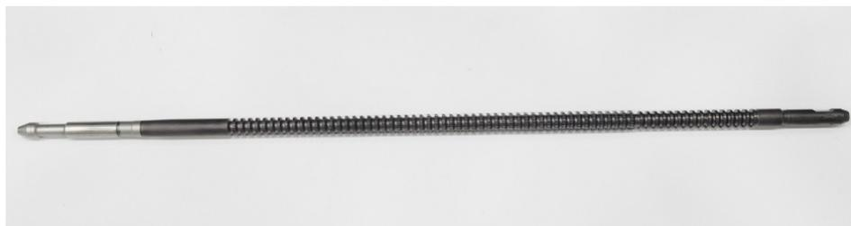
**Figure 12.** Model broach coated with **Type 1** and **Type 2** films.
