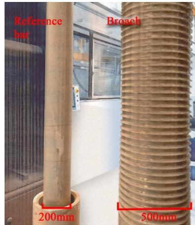
Figure 1. Outlining huge equipment dimensions and potential tool sizes.
