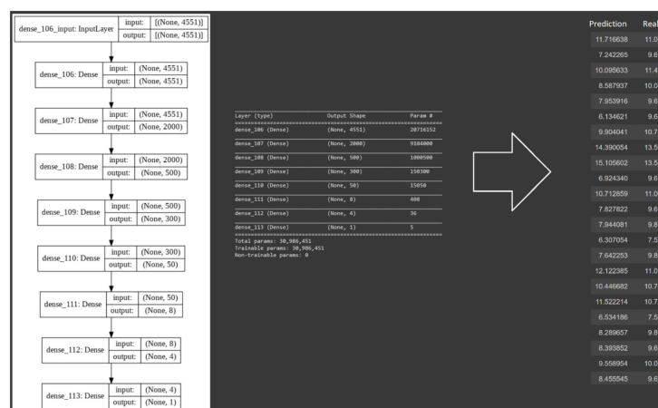
Figure 9. The structure of the neural network model designed for training with the spectral approach. The model is composed of eight dense layers. Layers 1 to 8 have 4551, 2000, 500, 300, 50, 8, 4 and 1 neuron/s, respectively, generating a total of over 30 million parameters requiring computation. The model's R^2 value is 0.153.
