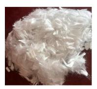
Figure 1. The polypropylene fibers.
