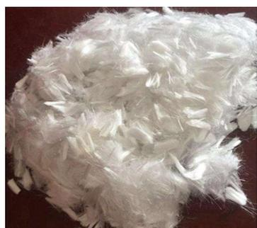
**Figure 1.** The polypropylene fibers.
