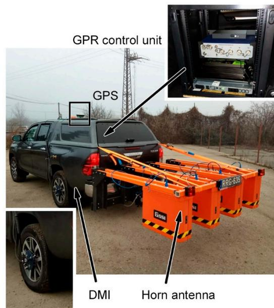
Figure 2. Main parts of the ground-penetrating radar (source: RODEN Engineering Office).
