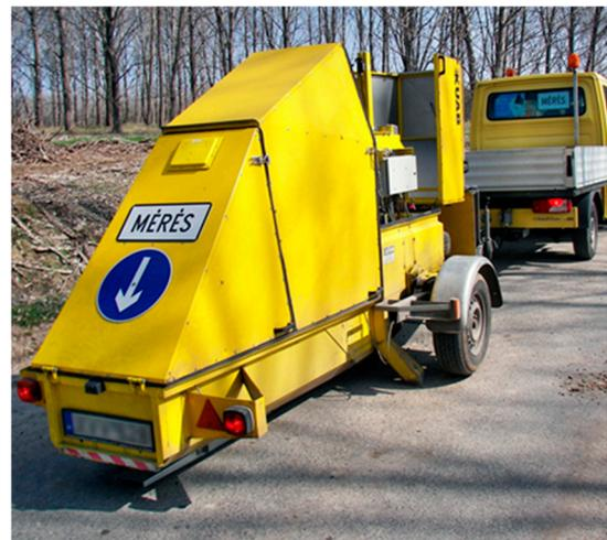
**Figure 1.** Schematic representation of FWD operation (left) and KUAB FWD testing equipment (right).
