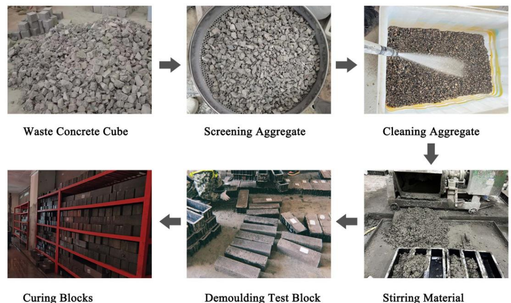
Figure 1. Test-block preparation and maintenance.
