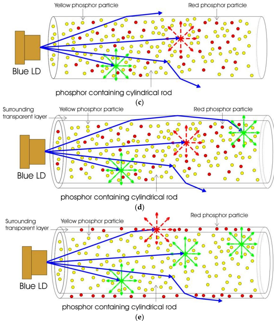
**Figure 1.** Schematic diagrams of (a) yellow phosphor cylindrical rod, (b) yellow phosphor cylindrical rod with surrounding transparent layer, (c) yellow and red phosphors cylindrical rod, (d) yellow and red phosphors cylindrical rod with surrounding transparent layer and (e) yellow cylindrical rod and surrounding red phosphor layer used in this study.
