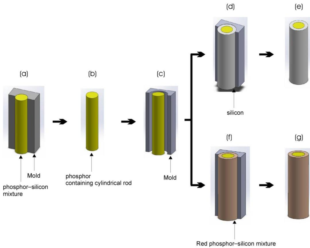
**Figure 2.** Schematic diagram of process flow charts in this study.
