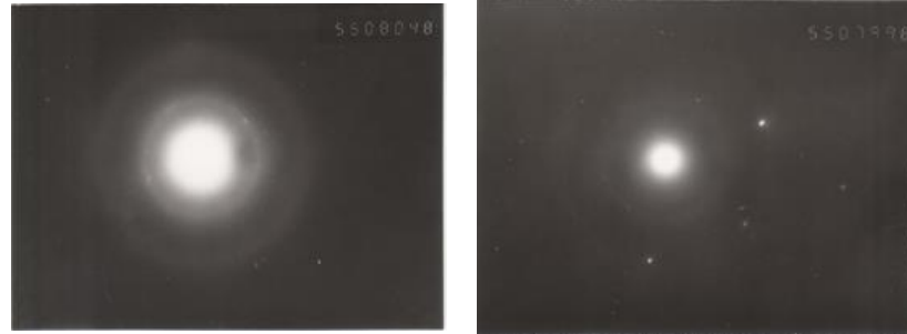
Figure 3. Nanodiamond X-ray diffraction pattern.
