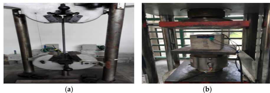
Figure 7. Steel bar and concrete materials tests: (a) Test rig for tensile strength of steel bar (HRB335); (b) Test rig for compressive strength of concrete.
