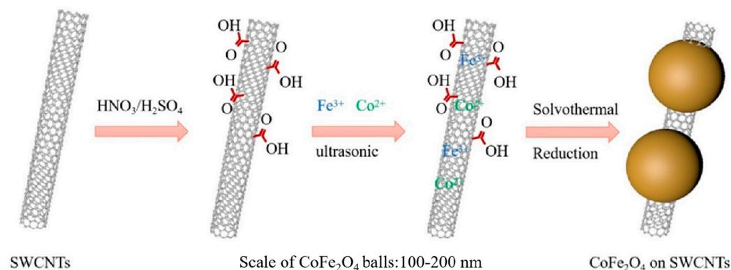
**Figure 1.** Schematic illustration of synthesis strategy for CoFe<sub>2</sub>O<sub>4</sub>/SWCNTs composites.
