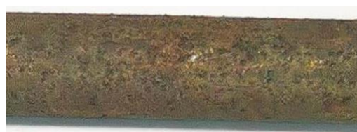
Figure 9. Macroscopic surface of corroded steel wire.
