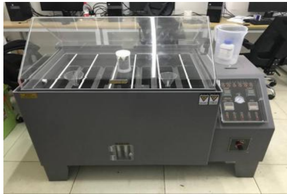
Figure 6. Salt fog corrosion chamber.
