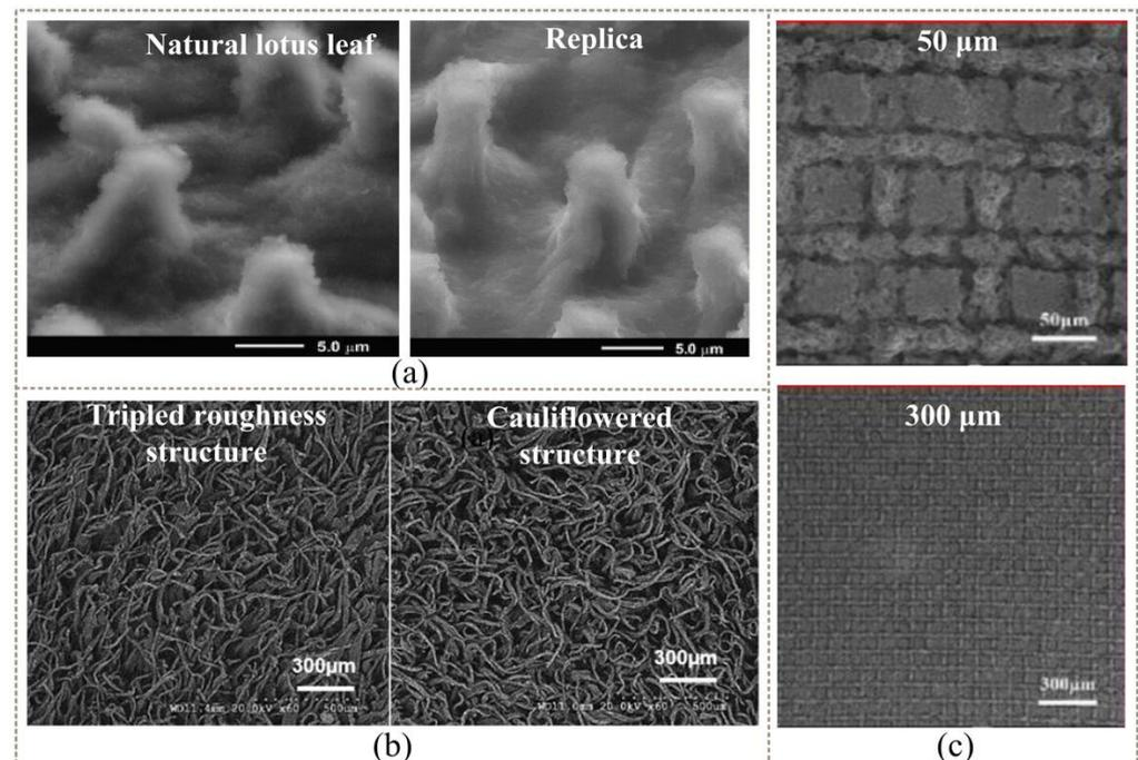
**Figure 3.** Preparation effects of the template method: (a) SEM images of the natural lotus leaf and its positive replica [53]; (b) SEM images of superoleophobic rough fibrous structures of high-density polyethylene (HDPE) [65]; (c) SEM images of the flexible tube [66].
