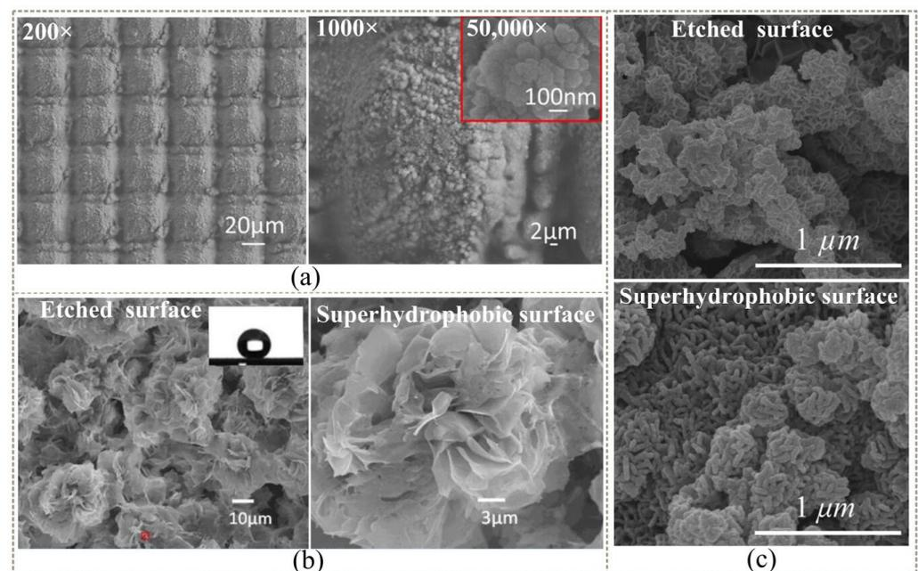
**Figure 5.** Preparation effects of etching methods: (a) SEM images of a superhydrophobic surface with cross-groove structures [63]; (b) SEM images of brass with a superhydrophobic surface [58]; (c) SEM images of the original surface, the etched surface, and the superhydrophobic surface [74].
