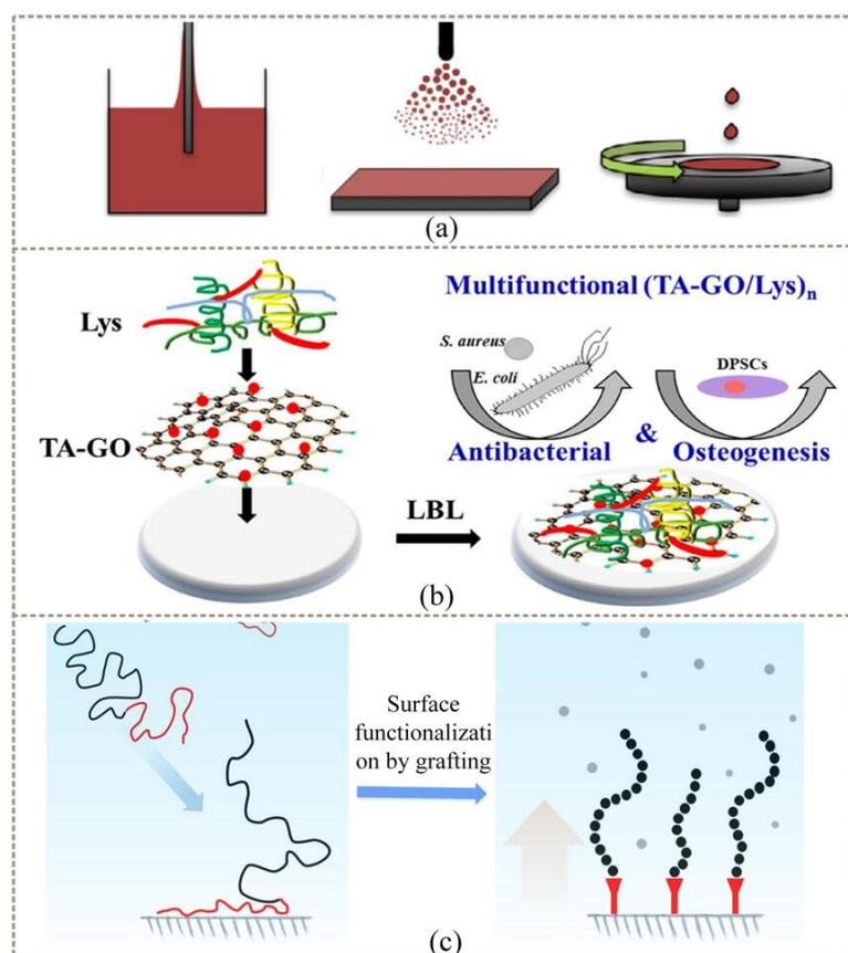
**Figure 7.** Different methods of attaching antibacterial coatings to material surfaces: (a) infiltrate, spray, and rotate [93]; (b) layer-by-layer self-assembly [94]; (c) surface grafting [95].
