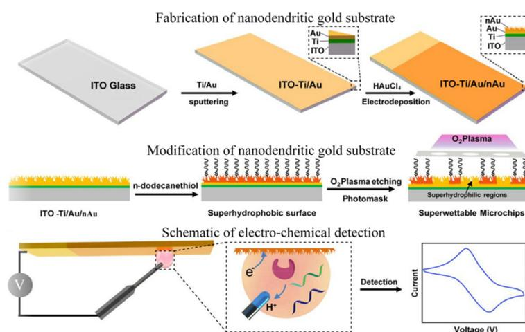
**Figure 13.** Design of ultra-wettable electrochemical microchips for biosensing [200].
