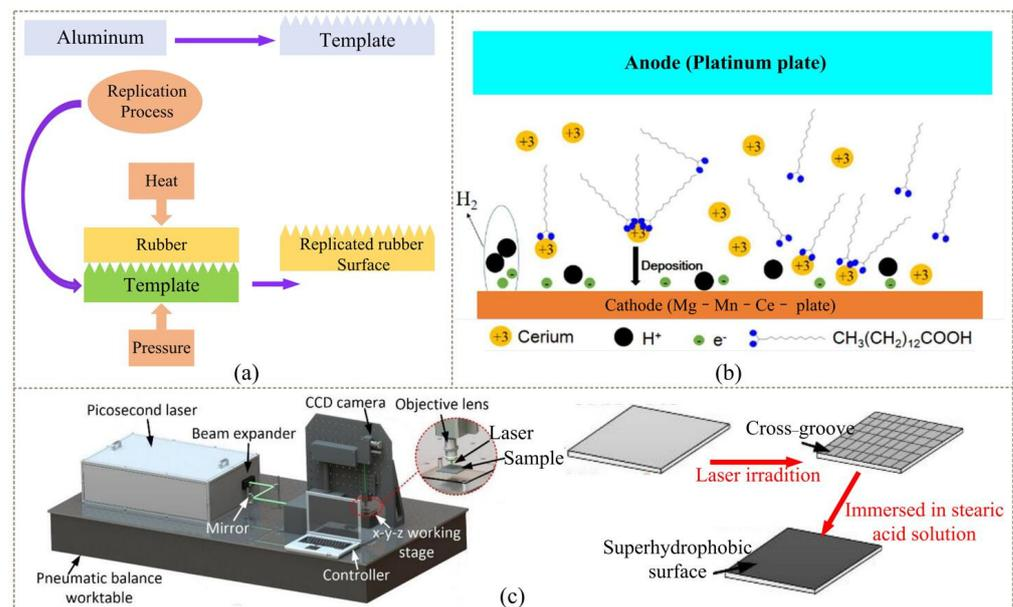
**Figure 2.** Preparation methods and principles of superhydrophobic surfaces: (a) template method [61]; (b) spraying method [62]; (c) etching method [63].
