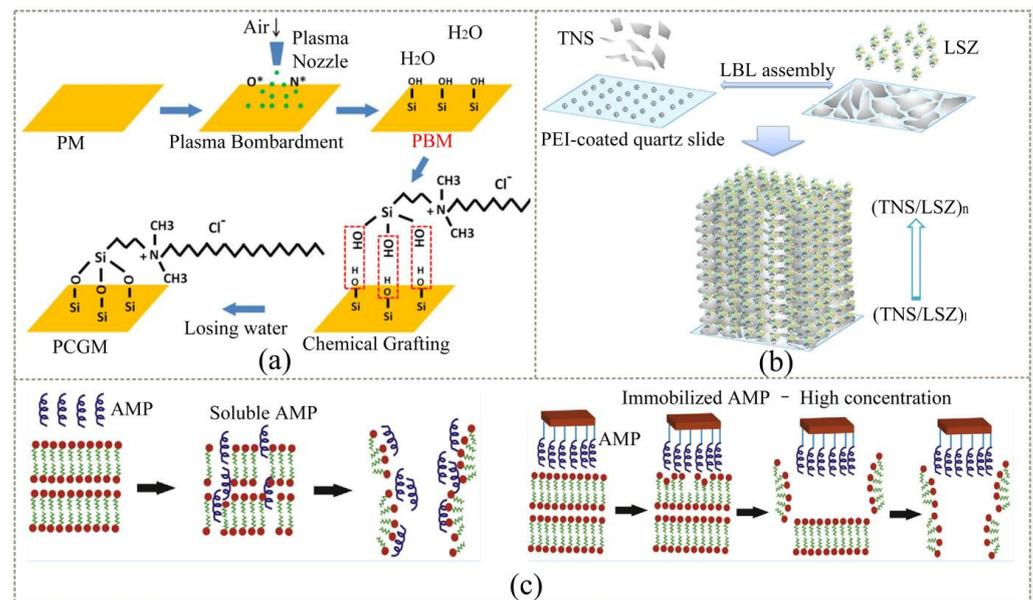
**Figure 8.** Preparation process and bactericidal mechanism of contact-type antibacterial coatings: (a) preparation of a glass-fiber membrane modified by QASs [101]; (b) schematic illustration of the procedure for fabricating the TiO<sub>2</sub> nanosheets (TNS)/lysozyme (LSZ) multilayer composite film [125]; (c) mechanism of action of immobilized CM against bacterial membranes [126].
