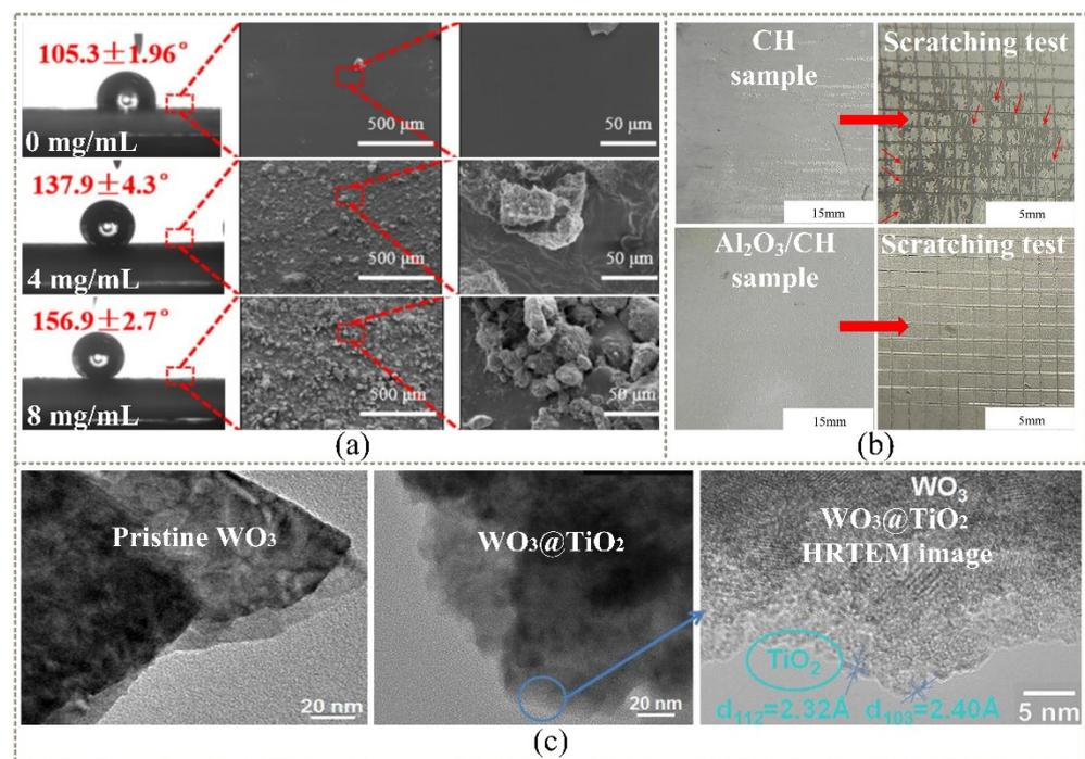
**Figure 4.** Preparation effects of the spraying methods: (a) effects of the content of carbon nanotube materials on coatings, non-wettability, and morphology [69]; (b) scratching methods to evaluate the adhesion strength of the layers [70]; (c) TEM images of pristine  $\text{WO}_3$  and  $\text{WO}_3@/\text{TiO}_2$  nanocomposite film [72].
