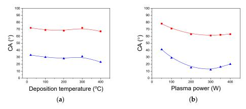
**Figure 16.** (a) Contact angles as function of deposition temperature (series B). (b) Contact angles as function of plasma power (series D). Test liquids are water (square) and diethylene glycol (triangle).
