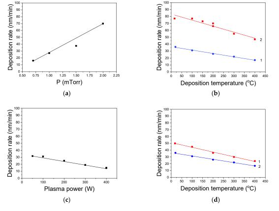
**Figure 1.** (a) Deposition rate of films versus TMDSN partial pressure (Series A); (b) Film growth rate as a function of the deposition temperature for TMDSN pressure of 1 mTorr (1) and 2 mTorr (2). (Series B and C); (c) Growth rate of films versus plasma power (Series D); (d) Temperature dependence of film growth rate for plasma power of 100 W (1) and 200 W (2). (Series E and B).
