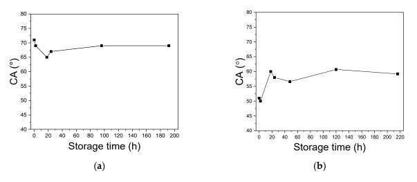
**Figure 18.** Time dependence of contact angles for films deposited using TMDSN + Ar (**a**) and TMDSN +  $N_2$  (**b**) mixture.
