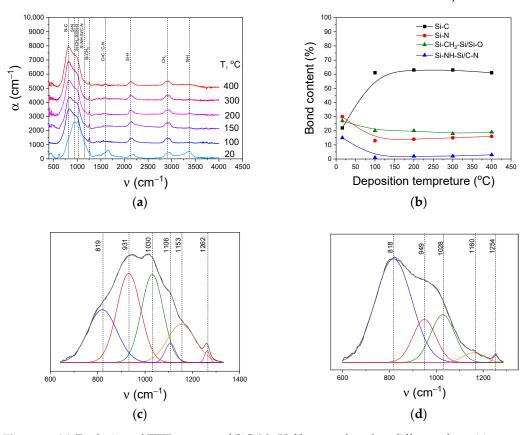
**Figure 7.** (a) Evolution of FTIR spectra of SiC<sub>x</sub>N<sub>y</sub>:H films produced at different deposition temperature (Series C); (b) The relative integrated intensities of the IR bands from the Si–N, Si–C, and Si–CH<sub>2</sub>–Si/Si–O units. Result of deconvolution into Gaussian profiles of the absorption band in the range of 1400–700 cm<sup>-1</sup> for SiC<sub>x</sub>N<sub>y</sub>:H films deposited at 20 °C (c) and 400 °C (d).
