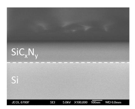
**Figure 4.** Cross-section SEM image of SiC<sub>x</sub>N<sub>y</sub>:H/Si(100) structure. The film deposition conditions:  $T_{dep} = 200 \degree C$ , W = 200 W, F(Ar) = 30 sccm, F(N<sub>2</sub>) = 0 sccm.
