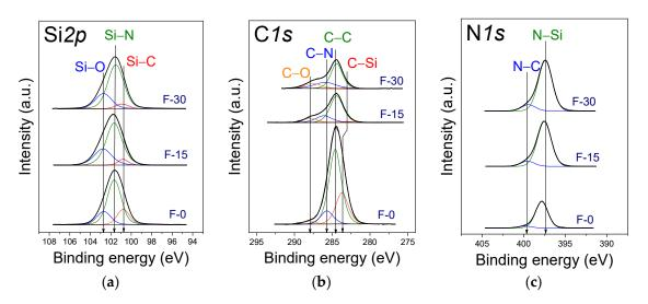
Figure 9. Si2p (a), C1s (b), and N1s (c) spectra of a-SiC<sub>x</sub>N<sub>v</sub>:H films.
