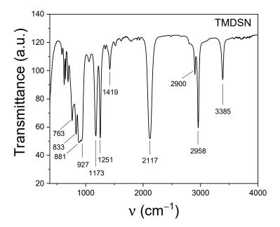
Figure 6. FTIR spectrum of TMDSN precursor.
