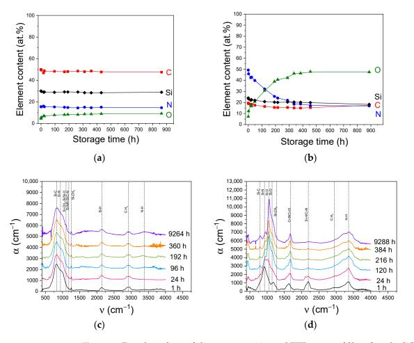
**Figure 17.** Time dependence of element composition and FTIR spectra of films. Samples SiCN-A (**a**,**c**) and SiCN-N (**b**,**d**).
