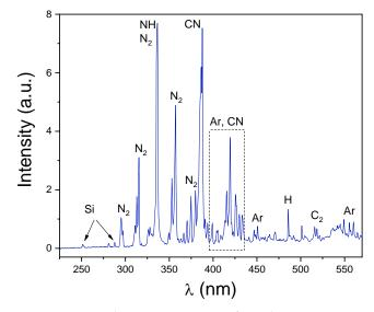
**Figure 10.** Optical emission spectrum from the TMDSN +  $Ar + N_2$  plasma. The spectrum has been measured on ICP CVD reactor with 200 W plasma power, 30 sccm total flow,  $R(N_2) = 0.54$ , and P(TMDSN) = 1 mTorr.
