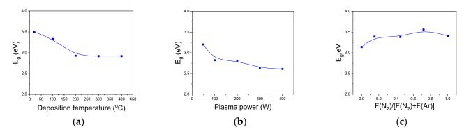
**Figure 15.** The optical band gap of  $SiC_xN_y$ :H films as function of (**a**) the deposition temperature (series B); (**b**) plasma power (series D); and (**c**) the value of the ratio  $R(N_2)$  (series F).
