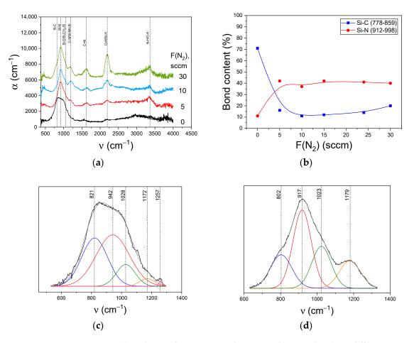
**Figure 8.** (a) Evolution of FTIR spectra of SiC<sub>x</sub>N<sub>y</sub>:H films produced at a different nitrogen flow rate (Series F); (b) The relative integrated intensities of the IR bands from the Si–N and Si–C units. Result of deconvolution into Gaussian profiles of the absorption band in the range of 1300–600 cm<sup>-1</sup> for SiC<sub>x</sub>N<sub>y</sub>:H films deposited at  $F(N_2) = 0$  (c) and 30 sccm (d).
