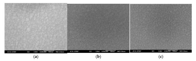
**Figure 3.** SEM images of SiC<sub>x</sub>N<sub>y</sub>:H deposited from TMDSN + N<sub>2</sub> mixture at  $F(N_2) = 0$  (**a**), 15 (**b**), and 30 (**c**) sccm.
