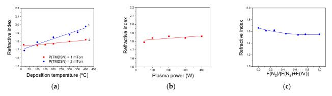
**Figure 13.** Refractive index of  $SiC_xN_y$ :H films as function of (**a**) the deposition temperature (series B and C); (**b**) plasma power (series D), and (**c**) the value of the ratio  $R(N_2)$  (series F).
