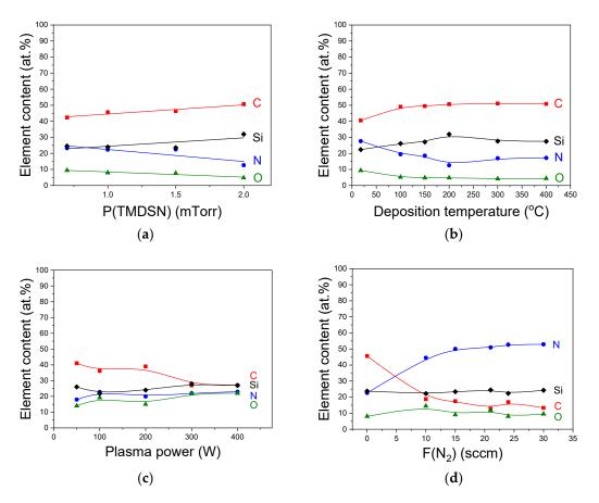
**Figure 5.** Elemental composition of  $SiC_xN_y$ :H films depending on TMDSN pressure (**a**); deposition temperature (**b**); plasma power (**c**); and nitrogen flow rate (**d**).
