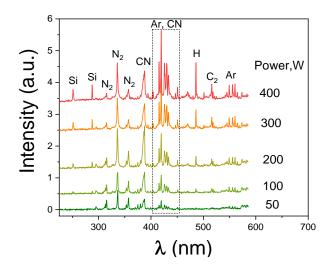
Figure 12. Emission spectra of TMDSN + Ar plasma at different RF discharge powers.
