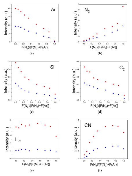
**Figure 11.** Dependences of the intensities of the argon line at 763.5 nm (**a**), the nitrogen N<sub>2</sub> band at 357 nm (**b**), the silicon line at 288.2 nm (**c**), the C<sub>2</sub> dimer band at 516.5 nm (**d**), the H $\alpha$  hydrogen line at 656.3 nm (**e**), the cyano radical CN band at 386.5 nm (**f**) versus the value of the ratio R(N<sub>2</sub>). Triangles—plasma power 200 W, circles—plasma power 400 W.
