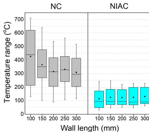
**Figure 13.** Comparison between temperature data distributions of walls built with different lengths under the NIAC (LEWD at 15 mm) and NC approaches.
