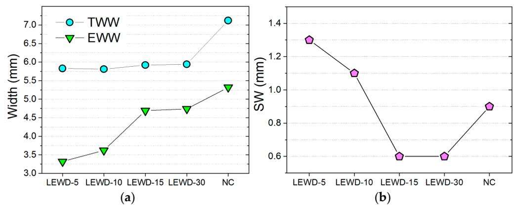
**Figure 6.** Quantitative effect of the LEWD parameter on the geometrical quality of the 350 mm-long walls: (a) effect of LEWD on the total and effective wall width and (b) on surface waviness.
