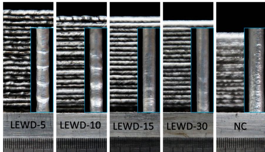
**Figure 4.** Effect of the LEWD parameter on the lateral and top superficial aspects of the 350 mm-long walls.
