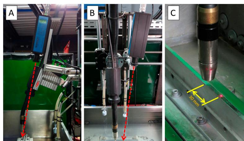
**Figure 2.** IR pyrometer arrangement for in-processing-measuring of the interpass temperature: (A) front view; (B) lateral view; (C) measuring spot target.
