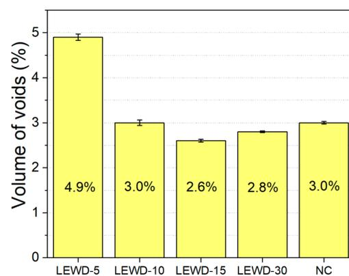
**Figure 7.** Effect of the LEWD parameter on the volume of voids of the 350 mm-long walls.
