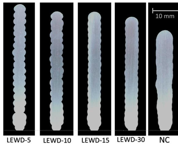
**Figure 5.** Qualitative effect of the LEWD parameter on the geometrical quality of the 350 mm-long walls.
