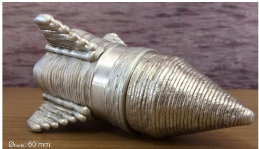
**Figure 1.** Thin-walled part of ER-5356 continuously deposited by WAAM with proper thermal management (Near-immersion Active Cooling technique as developed by da Silva et al. [6]) during preliminary tests (the continuous deposition, especially of the nose cone, would not be possible without proper thermal management due to the intense deposition concentration and consequent heat accumulation).
