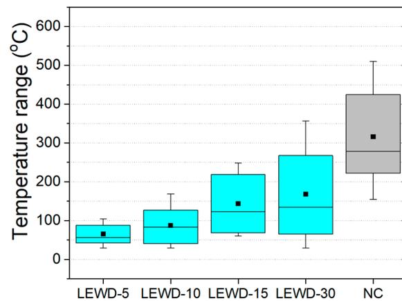
**Figure 10.** Effect of the LEWD parameter on the thermal features measured with the trailing/leading IR pyrometer in the 350 mm-long walls.
