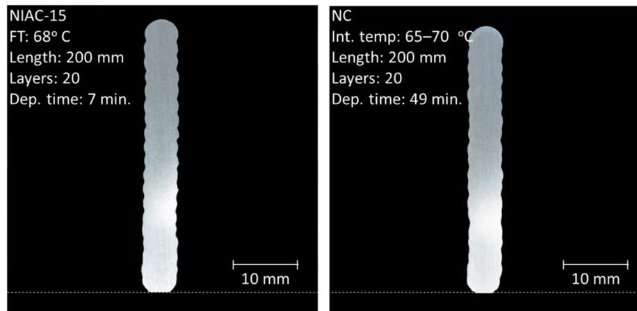
**Figure 11.** Comparison between 200 mm-long walls deposited with the NIAC and the NC approaches under equivalent interpass temperatures.
