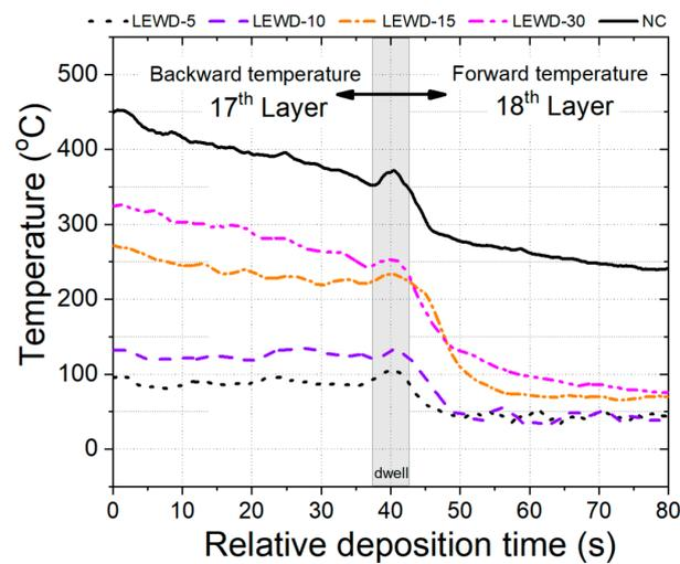
**Figure 8.** Temperature data from the trailing/leading IR pyrometer (after the deposition of 2 layers) of the 350 mm-long walls.
