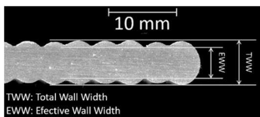
**Figure 3.** Geometrical features measured to characterize the surface texture of the walls [20].
