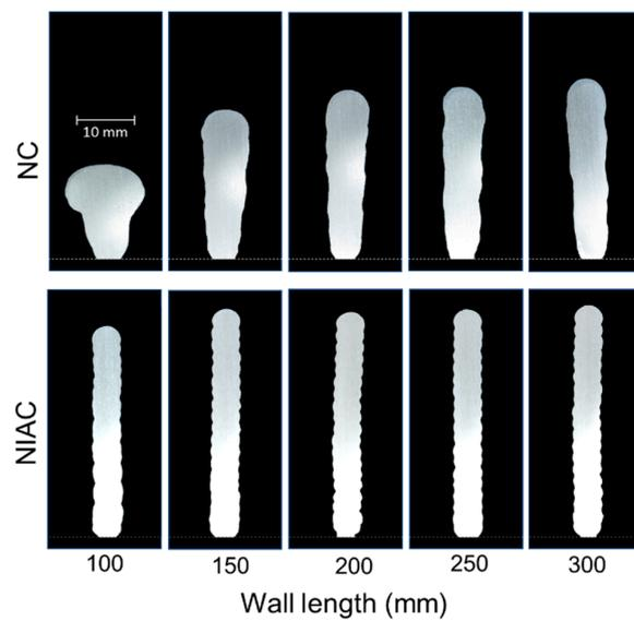
**Figure 12.** Effect of the deposition concentration on the geometry of walls with different lengths deposited with the NIAC (LEWD at 15 mm) and NC approaches.
