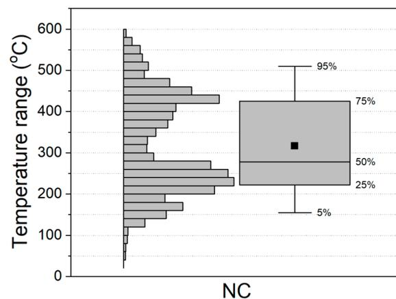
**Figure 9.** Temperature distribution based on the data acquired from the trailing/leading IR pyrometer during all the deposition time of a 300 mm-long wall with NC approached.
