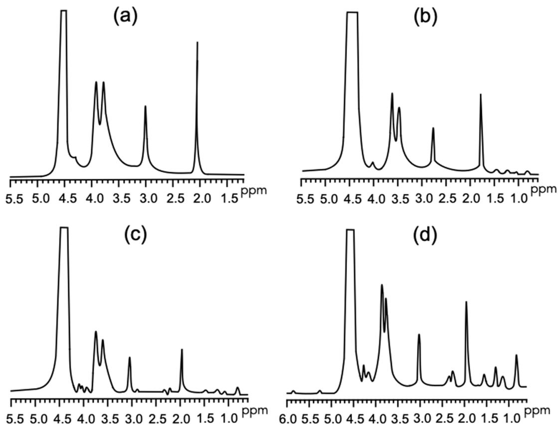
**Figure 5.**  $^1\text{H}$  NMR spectra of chitosan (CH) and squid gelatin hydrolysates (SGH) films: (a) 100 CH/ 0 SGH, (b) 90 CH/10 SGH, (c) 80 CH/20 SGH, and (d) 60 CH/40 SGH.
