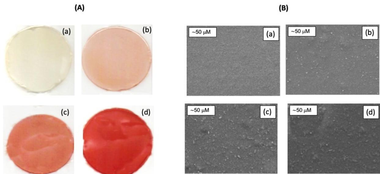
**Figure 2.** Photograph (A) and SEM images of the morphologies of the chitosan (CH) and squid gelatin hydrolysates (SGH) films at 1000× magnification (B): (a) 100 CH/0 SGH, (b) 90 CH/10 SGH, (c) 80 CH/20 SGH, and (d) 60 CH/40 SGH.
