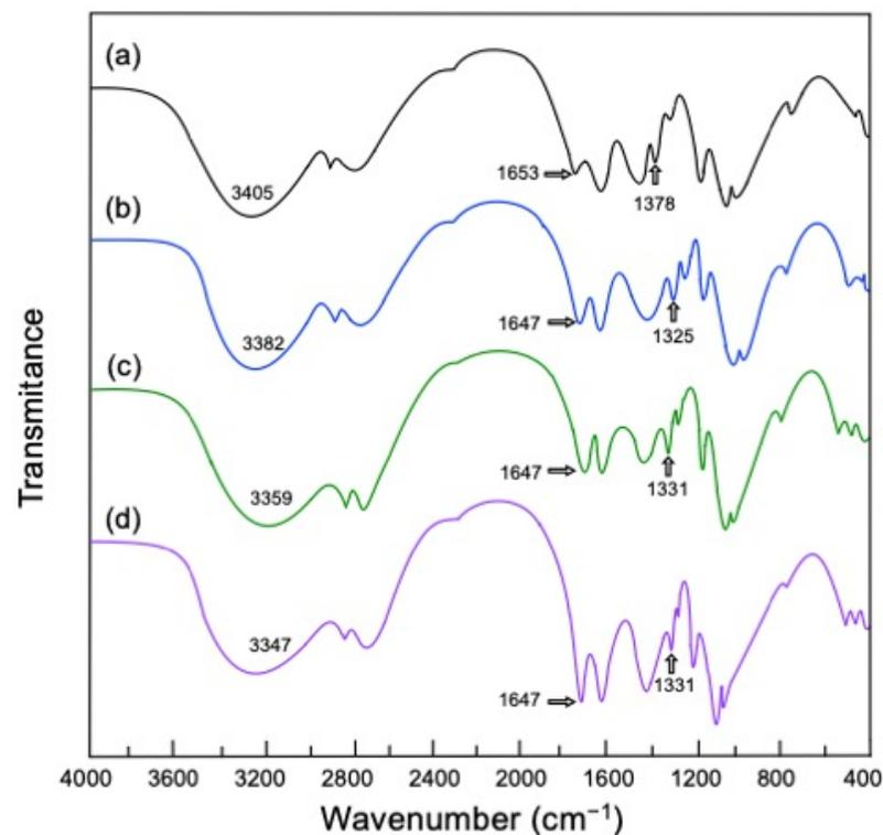
**Figure 4.** FT-IR spectra of chitosan (CH) and squid gelatin hydrolysates (SGH) films: (a)—100 CH/0 SGH, (b)—90 CH/10 SGH, (c)—80 CH/20 SGH, and (d)—60 CH/40 SGH.
