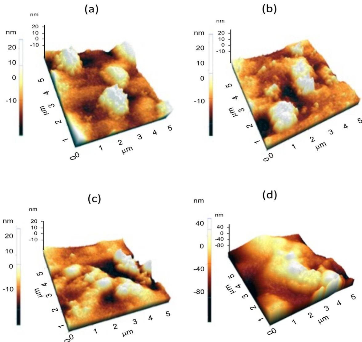
**Figure 3.** Images of the morphologies of chitosan (CH) and squid gelatin hydrolysates (SGH) films at 1000 $\times$  magnification: (a) 100 CH/0 SGH, (b) 90 CH/10 SGH, (c) 80 CH/20 SGH, and (d) 60 CH/40 SGH.
