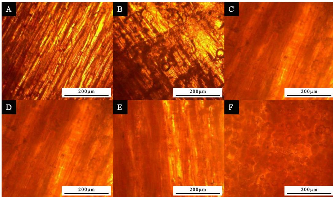
**Figure 3.** Microstructure of paint film with different contents of nano-silver solution: (A) 1.0%, (B) 4.0%, (C) 7.0%, (D) 10.0%, (E) 13.0%, and (F) 16.0%.
