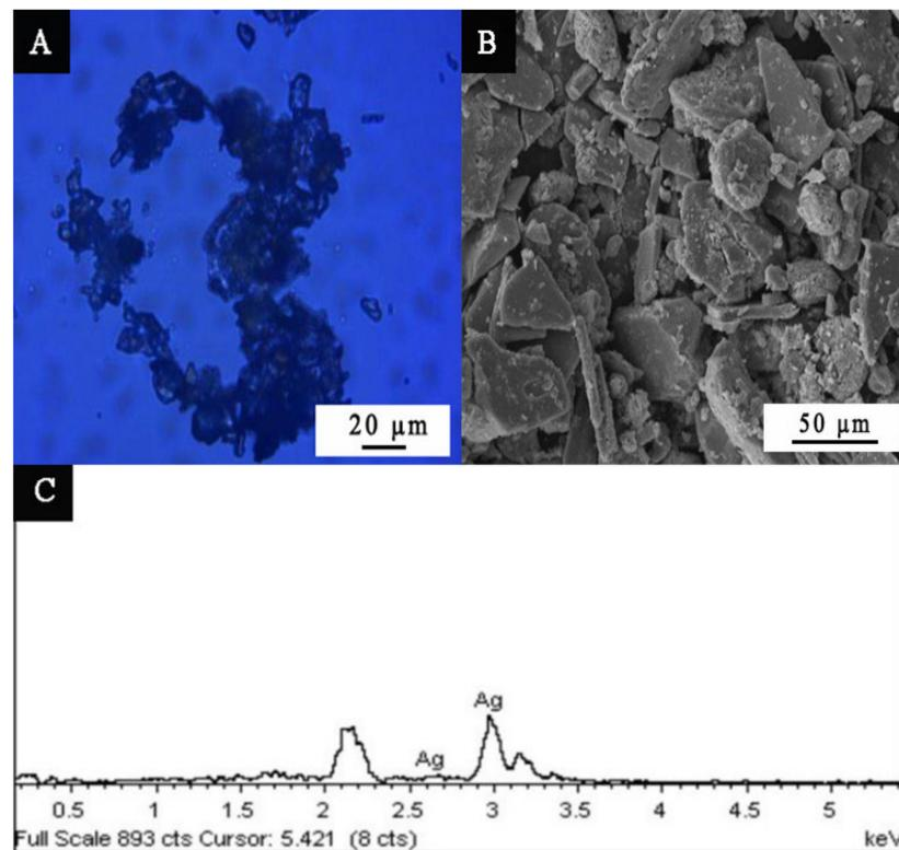
**Figure 1.** (A) OM image of micron silver particles, (B) SEM microscopic morphology of micron silver particles, and (C) EDS of micron silver particles.
