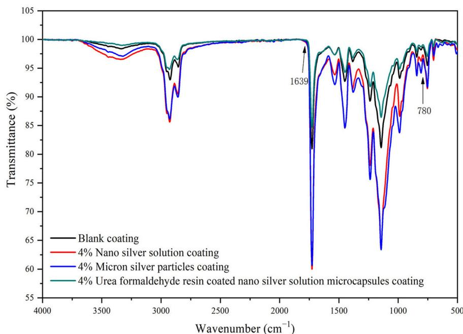
**Figure 7.** Infrared spectrum of paint film with 4.0% micron silver particles, 4.0% nano-silver solution, and 4.0% urea formaldehyde resin coated nano-silver solution microcapsules.
