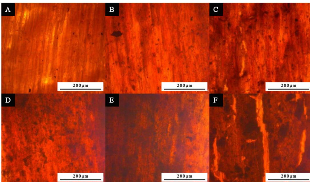
**Figure 4.** Microstructure of paint film with different contents of micron silver particles: (A) 1.0%, (B) 4.0%, (C) 7.0%, (D) 10.0%, (E) 13.0%, and (F) 16.0%.
