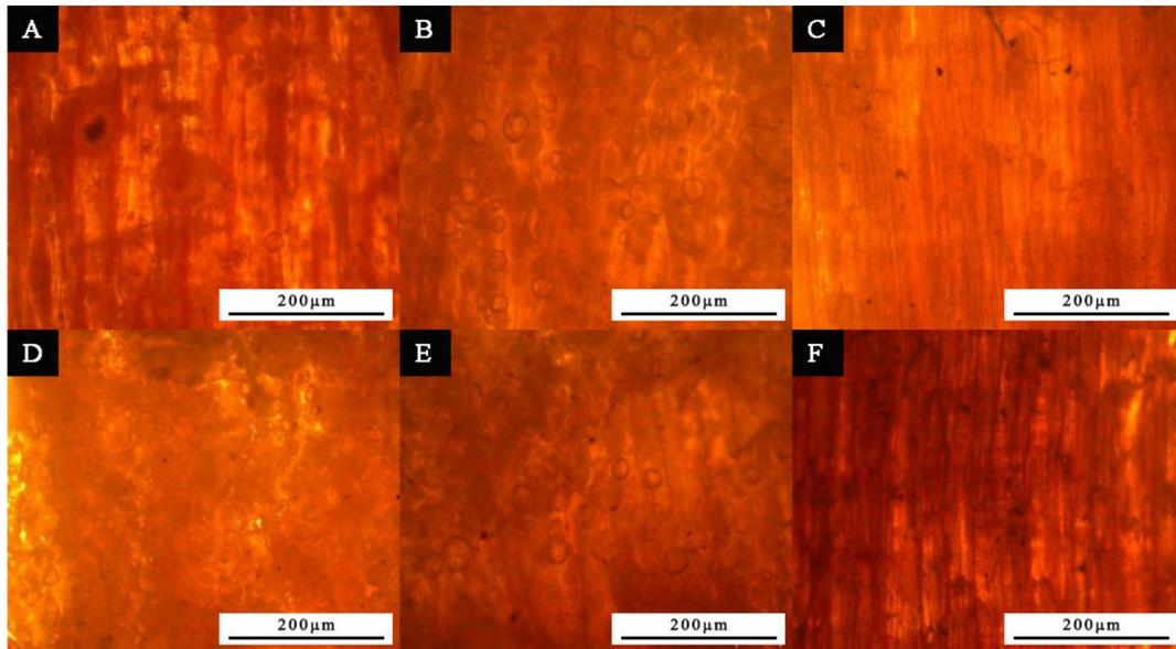
**Figure 5.** Microstructure of paint film with different contents of urea formaldehyde resin-coated nano-silver solution microcapsules: (A) 1.0%, (B) 4.0%, (C) 7.0%, (D) 10.0%, (E) 13.0%, and (F) 16.0%.
