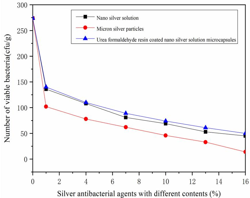
Figure 8. Number of surviving colonies in the coating with micron silver particles, nano-silver solution, and urea formaldehyde resin-coated nano-silver solution microcapsules.
