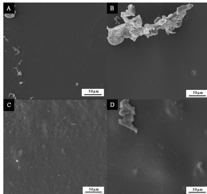
**Figure 6.** SEM image of paint film: (A) without silver antibacterial agents, (B) with 4.0% of nano-silver solution, (C) with 4.0% of micron silver particles, and (D) with 4.0% of urea formaldehyde coated nano-silver solution microcapsules.
