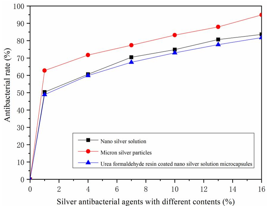
Figure 9. Antibacterial rate of the coating added with micron silver particles, nano-silver solution, and urea formaldehyde resin-coated nano-silver solution microcapsules.
