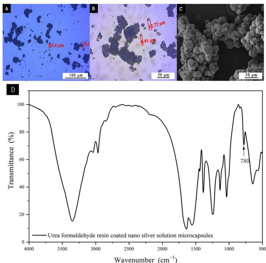
**Figure 2.** OM of urea formaldehyde resin-coated nano-silver solution microcapsules: (A) under 10× objective lens and (B) under 20× objective lens. (C) SEM microscopic view of urea formaldehyde resin-coated nano-silver solution microcapsules and (D) infrared spectrum of urea-formaldehyde resin-coated nano-silver solution microcapsules.
