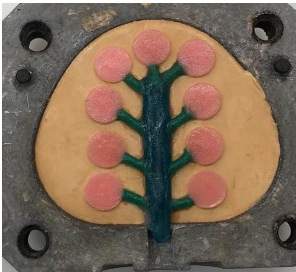
Figure 3. Wax patterns invested for injection molding technique.
