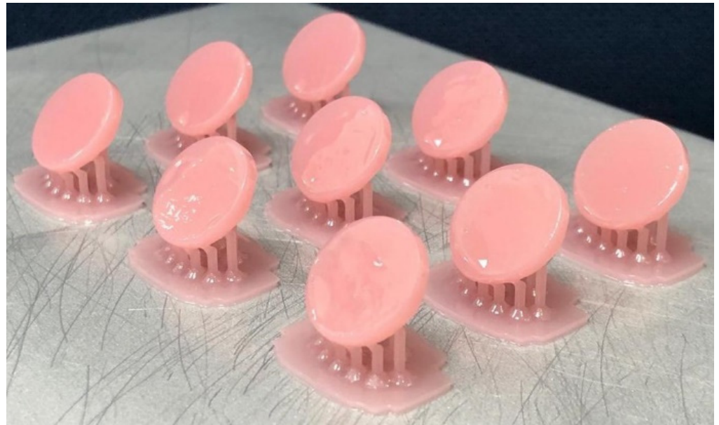
Figure 1. Specimens prepared by CAD/CAM additive manufacturing technique (3D printing).
