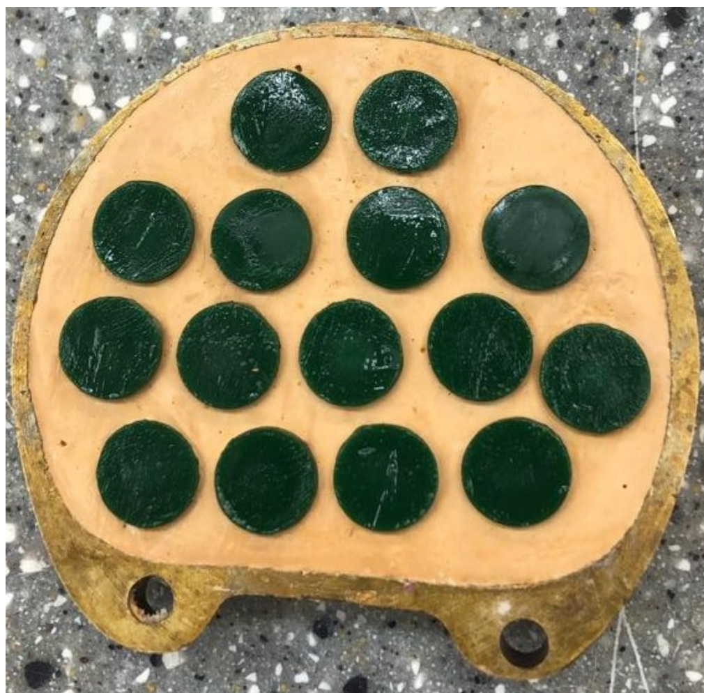
Figure 4. Wax patterns invested for conventional compression molding technique.
