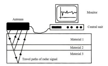
Figure 13. The basic configuration of ground-penetrating radar [62].
