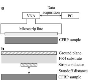
Figure 10. Detection system with microstrip line sensor (a) experiment setup (b) cross-section [56].
