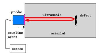
Figure 1. Basic principle of ultrasonic testing [22].
