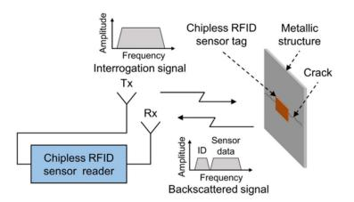
**Figure 7.** Basic principle of a chipless radio-frequency identification (RFID) sensor system for crack detection and characterization on a metallic structure [38].
