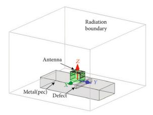
Figure 8. Simulation process of 3D RFID tag antenna on the metal structures with defects [50].
