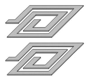
Figure 15. Vertical coupling of two spiral inductors [48].
