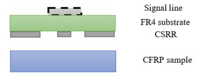
Figure 11. Side view of the complementary split-ring resonator (CSRR) [43].
