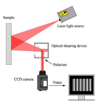
Figure 5. Setup system of laser shearography (LS) [14].
