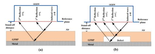
**Figure 12.** Cross-section diagram of the scanning arrangement using an open-ended rectangular waveguide in case of (**a**) defect-free and (**b**) defect [11].
