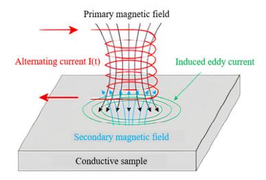
Figure 3. Induced currents in conductive material [32].
