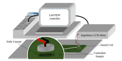
Figure 4. Schematic diagram of eddy current testing [33].
