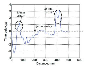
Figure 17. Time delay of all signals along with the scanning onto the materials using cross-correlation [75].
