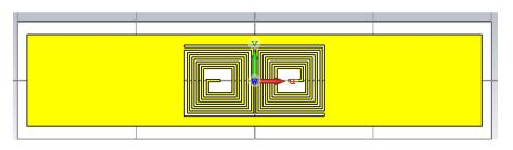
Figure 14. Planar coupling between two side-by-side spiral inductors.
