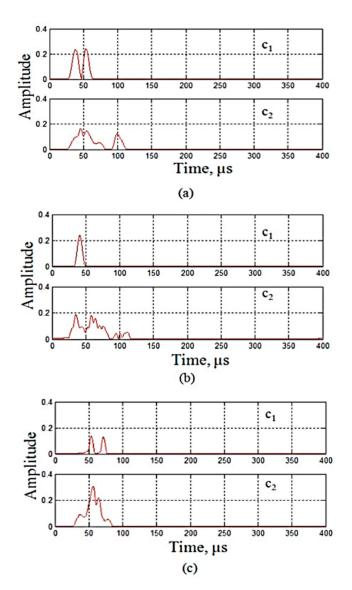
**Figure 18.** Instantaneous amplitudes of first two intrinsic mode functions (IMFs) using Hilbert transform (**a**) defect-free signal, (**b**) 15 mm defective signal, (**c**) 25 mm defective signal [75].
