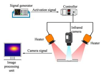
Figure 2. Setup of infrared thermography (IRT) [14].
