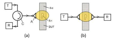
Figure 6. Microwave testing in (a) reflection mode and (b) transmission mode [37].
