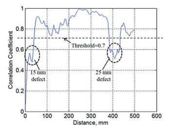
Figure 16. Correlation coefficient along with the scanning onto the materials using cross-correlation [75].
