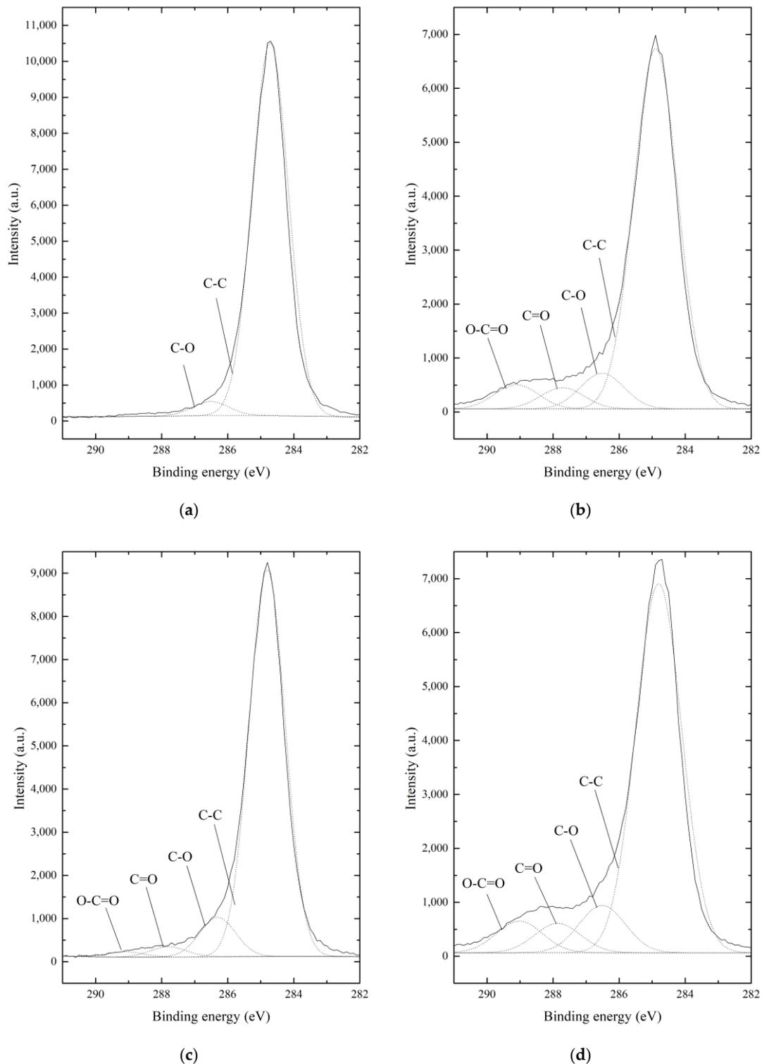
**Figure 13.** C1s spectra of the PE surface after being treated by (a) none, (b) APPJ only, (c) sanding only, and (d) both sanding and APPJ.
