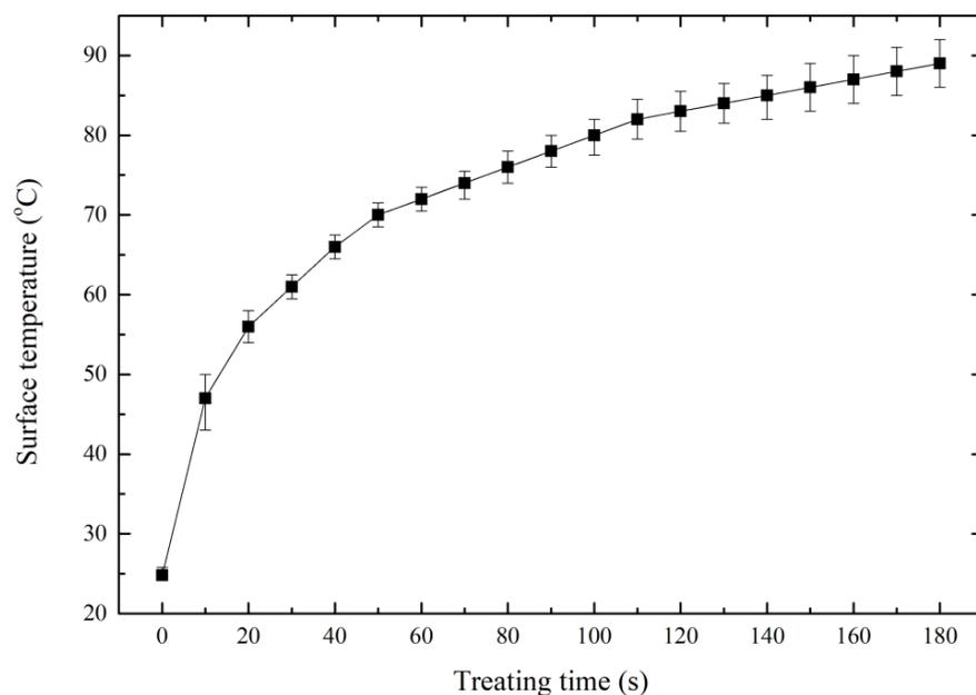
**Figure 5.** Surface temperature on the PP surface after various plasma treatment times. The thermal camera measured similar surface temperature during treatment time distribution for PET and PE.
