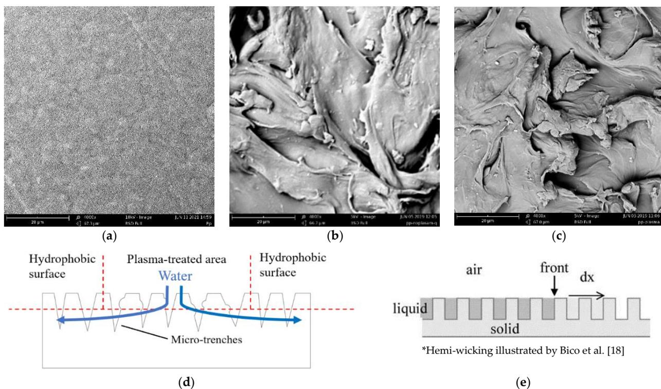
**Figure 7.** (a) SEM micrograph of untreated PP surface, (b) SEM micrograph of sanded PP surface, (c) SEM micrograph of PP surface treated by sanding and then plasma, (d) diagram of hemi-wicking phenomena on the sanded surface applied by the plasma activation, and (e) diagram of hemi-wicking phenomena illustrated in the prior study.
