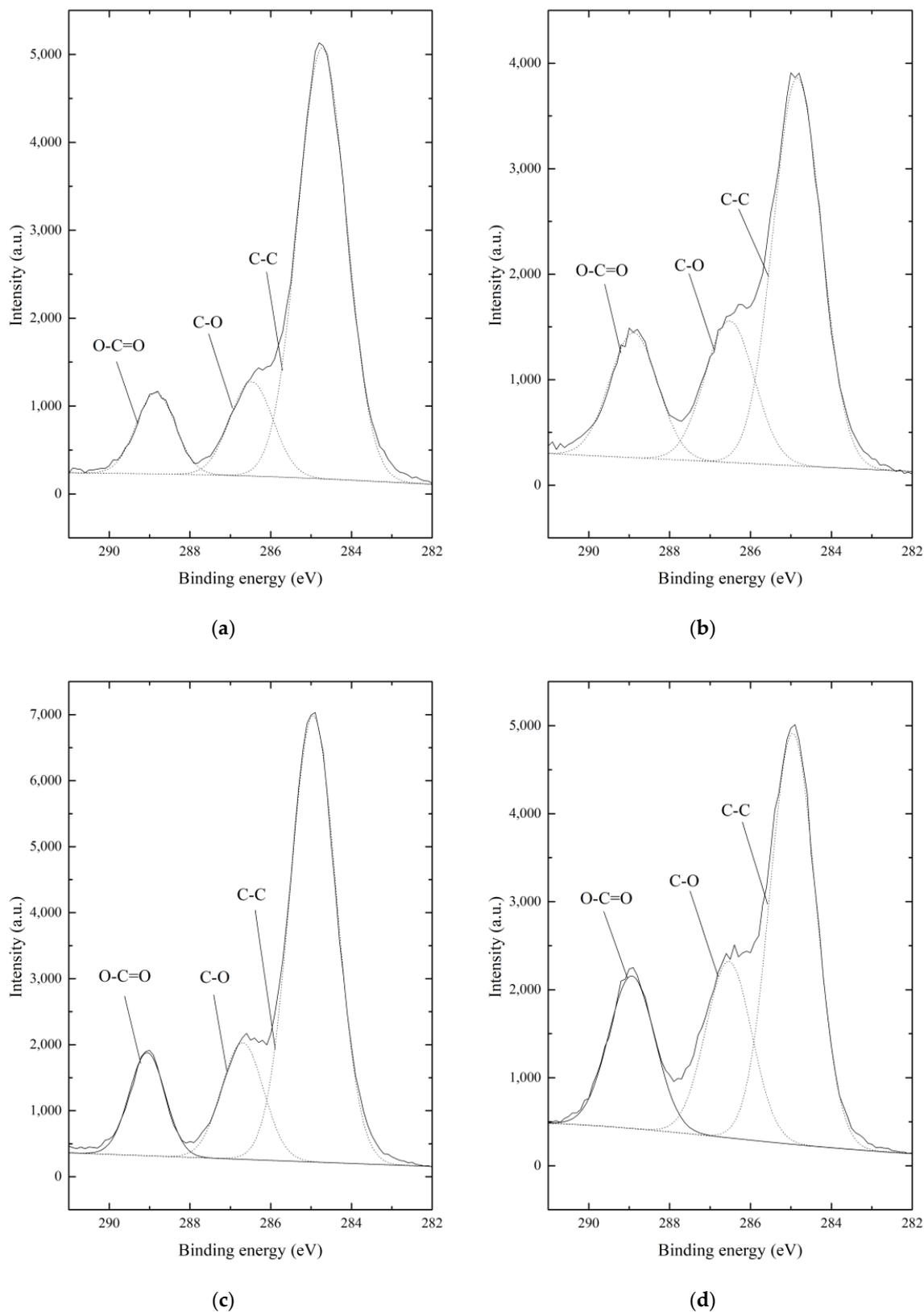
**Figure 12.** C1s spectra of the PET surface after being treated by (a) none, (b) APPJ only, (c) sanding only, and (d) both sanding and APPJ.
