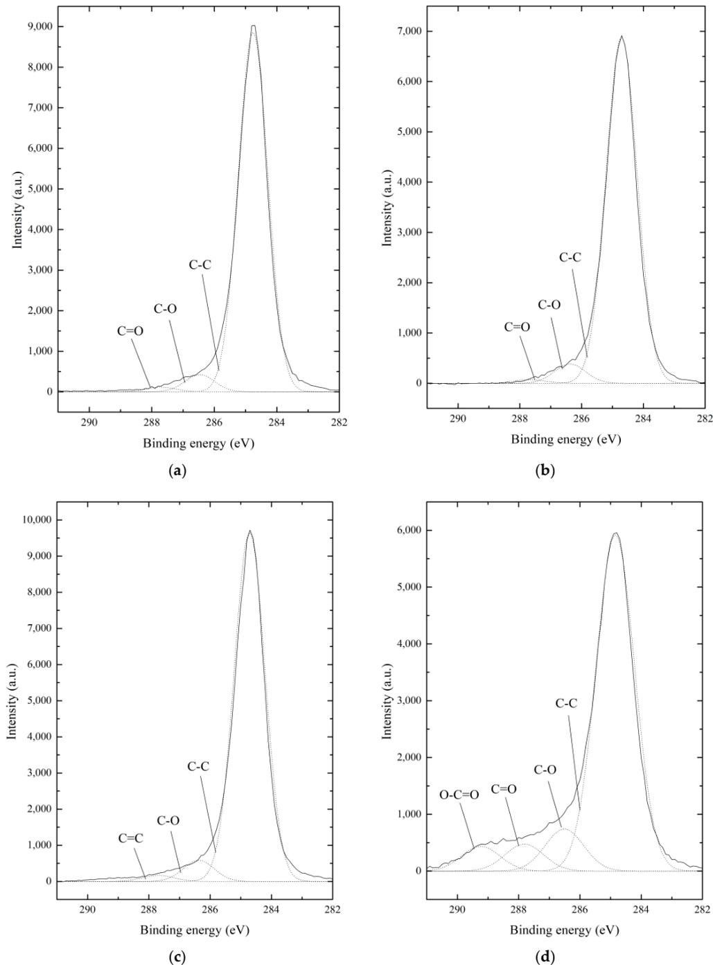
**Figure 11.** C1s spectra of the PP surface after being treated by (a) none, (b) APPJ only, (c) sanding only, and (d) both sanding and APPJ.
