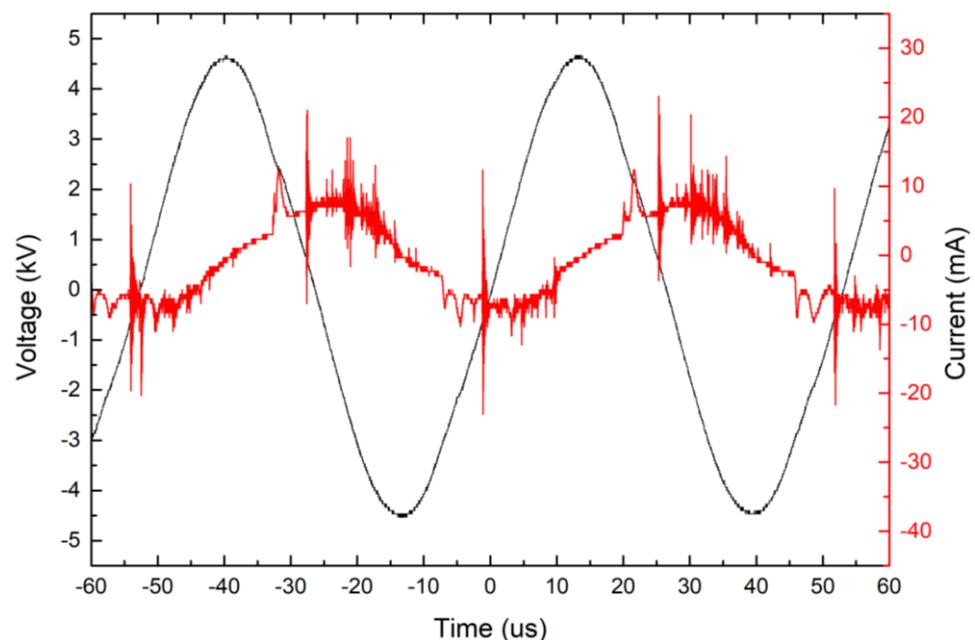
Figure 2. Typical current and voltage waveforms for the APPJ.
