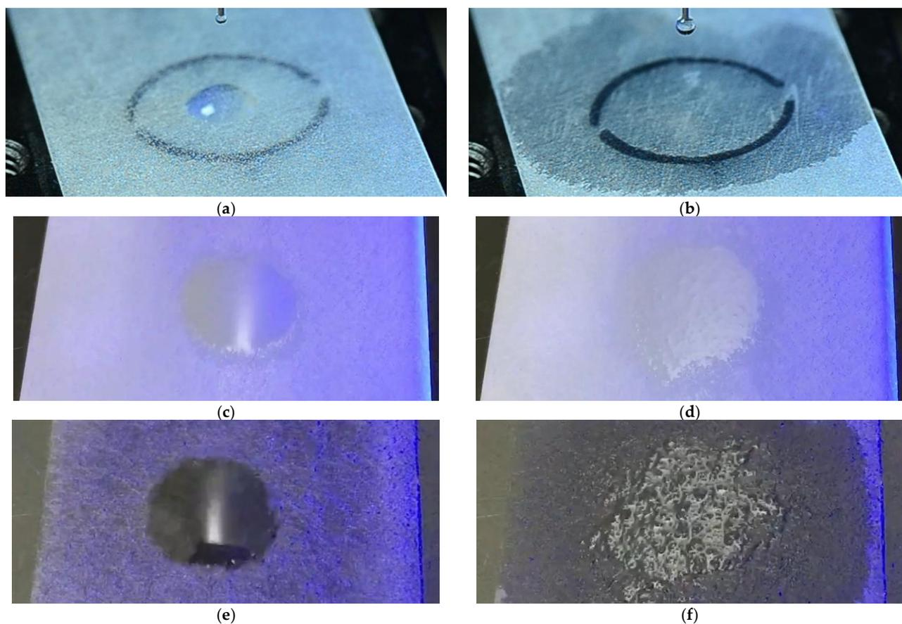
**Figure 6.** Snapshots for sanded films taken after being treated with APPJ at the moments that (a) a droplet was falling on a PP film initially; (b) the drop was spreading over the PP film; (c) a droplet was falling on a PET film initially; (d) the drop was spreading over the PET film; (e) a droplet was falling on a PE film initially; and (f) the drop was spreading over the PE film.
