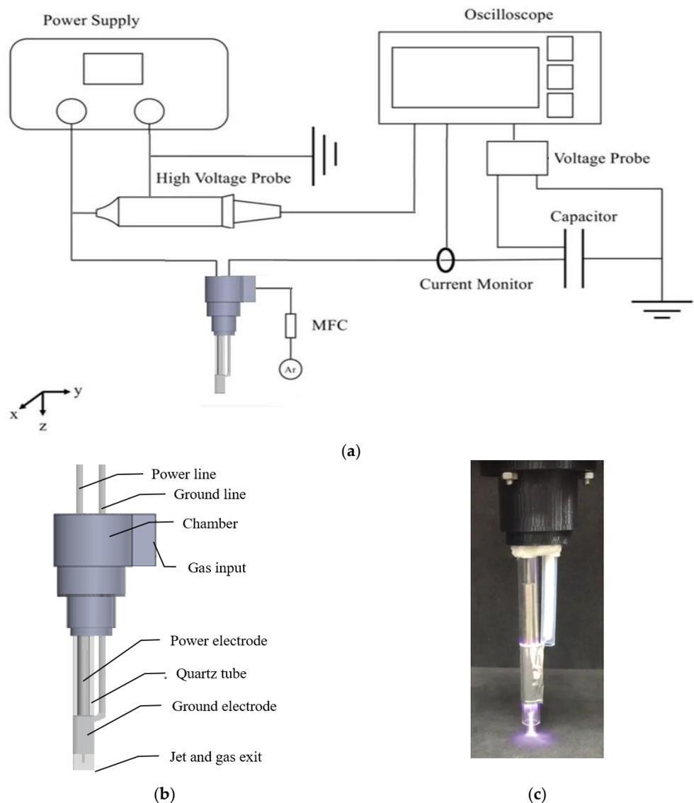
**Figure 1.** (a) Schematic of system including an APPJ device and electrical measurement devices; (b) schematic of the APPJ device; and (c) snapshot of the APPJ device with the generated plasma jet.
