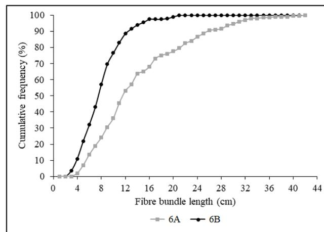
**Figure 2.** Frequency distribution curve of the length of fibre bundles extracted from batch number 6 using the A and B extracting methodologies.
