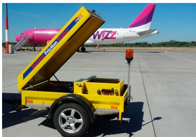
Figure 2. Airport Surface Friction Tester on Trailer T-10.
