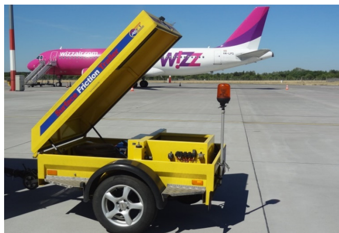
Figure 2. Airport Surface Friction Tester on Trailer T-10.
