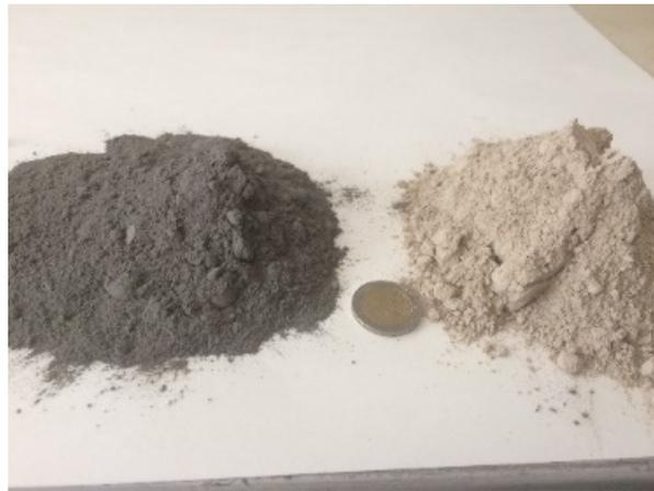
**Figure 2.** Limestone filler vs. jet grouting waste as filler.
