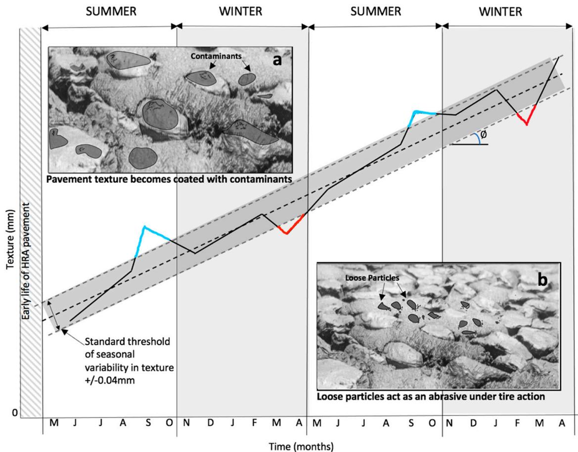
**Figure 9.** The governing trends of long-term change to pavement texture on hot rolled asphalt (HRA) pavement surface. (a) During the summer season pavement texture can become coated with contaminants such as the residue of rubber or rubber particles from vehicle tires, oils or auto lubricants. (b) During the winter season frost shattering in pavement microcracks, leads to loose particles, which can act as an abrasive under tires, polishing the pavement surface.
