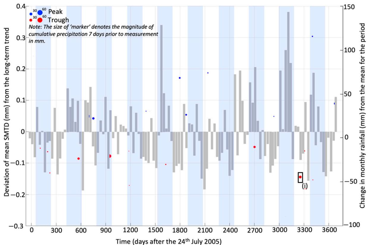
**Figure 8.** The graph plots change from mean monthly rainfall for the period 24 July 2005 to 1 August 2015, against the “peaks” and “troughs” in the deviation of mean SMTD for the southern sites on the A1. (See text for full explanation).
