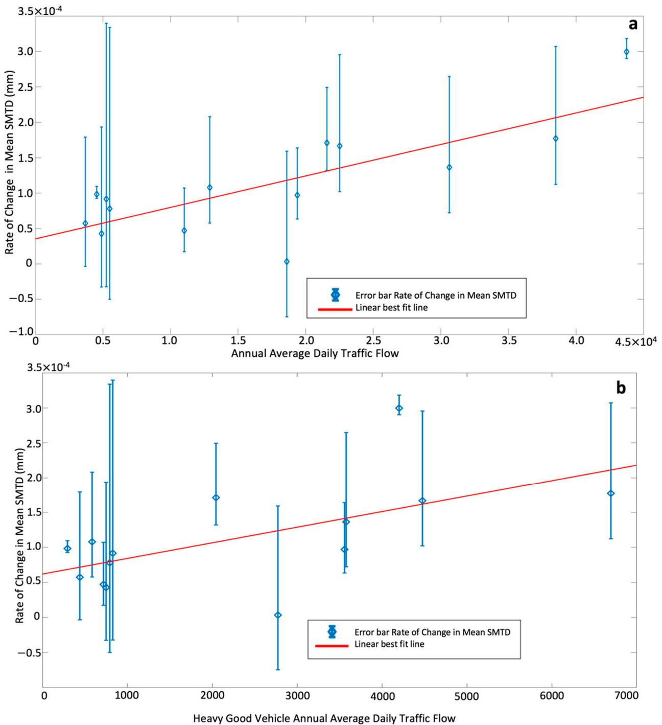
**Figure 4.** (a) Rate of change in mean sensor measured texture depth (SMTD) data compared with annual average daily traffic flow (AADT). (b) Rate of change in SMTD compared with heavy goods vehicle (HGV) AADT.
