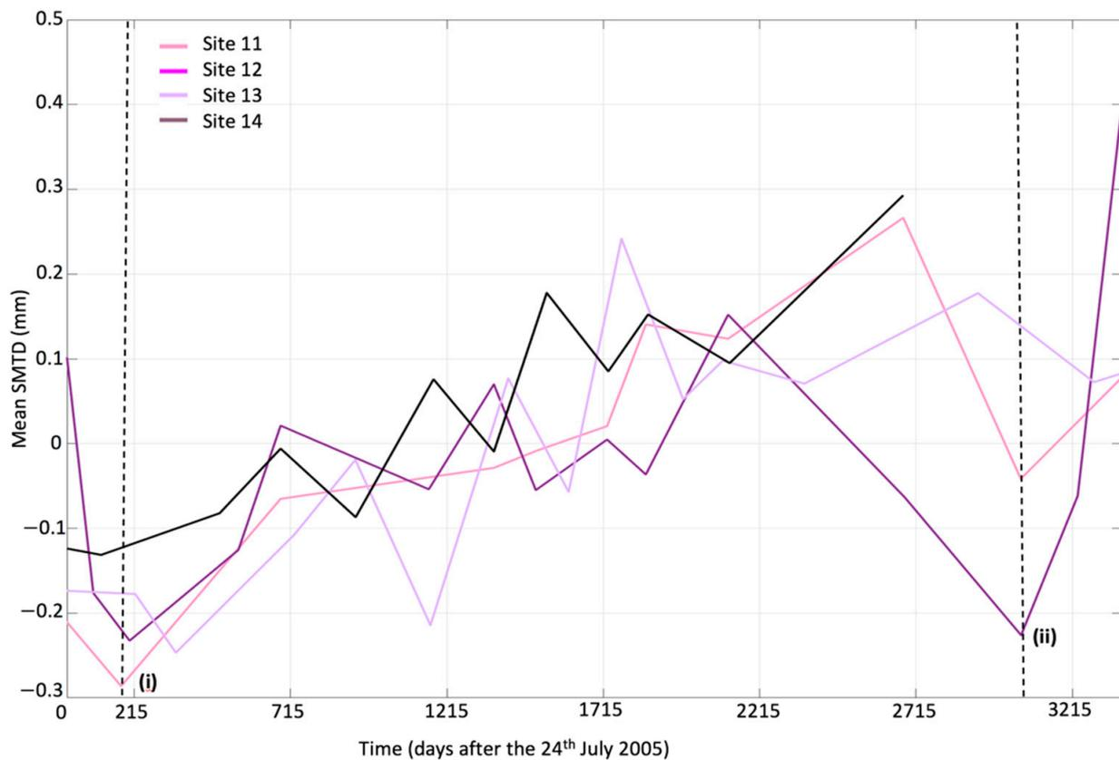
**Figure 3.** Normalised mean sensor measured texture depth (SMTD) data for the southern sites on the A1. (i) and (ii) are “troughs” in data coinciding with severe rainfall events. (See text for further explanation).
