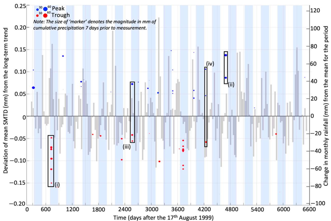
**Figure 7.** The graph plots change from mean monthly rainfall for the period 17 August 1999 to 17 July 2016, against the “peaks” and “troughs” in the deviation of mean SMTD for the northern sites on the A1. (See text for full explanation).
