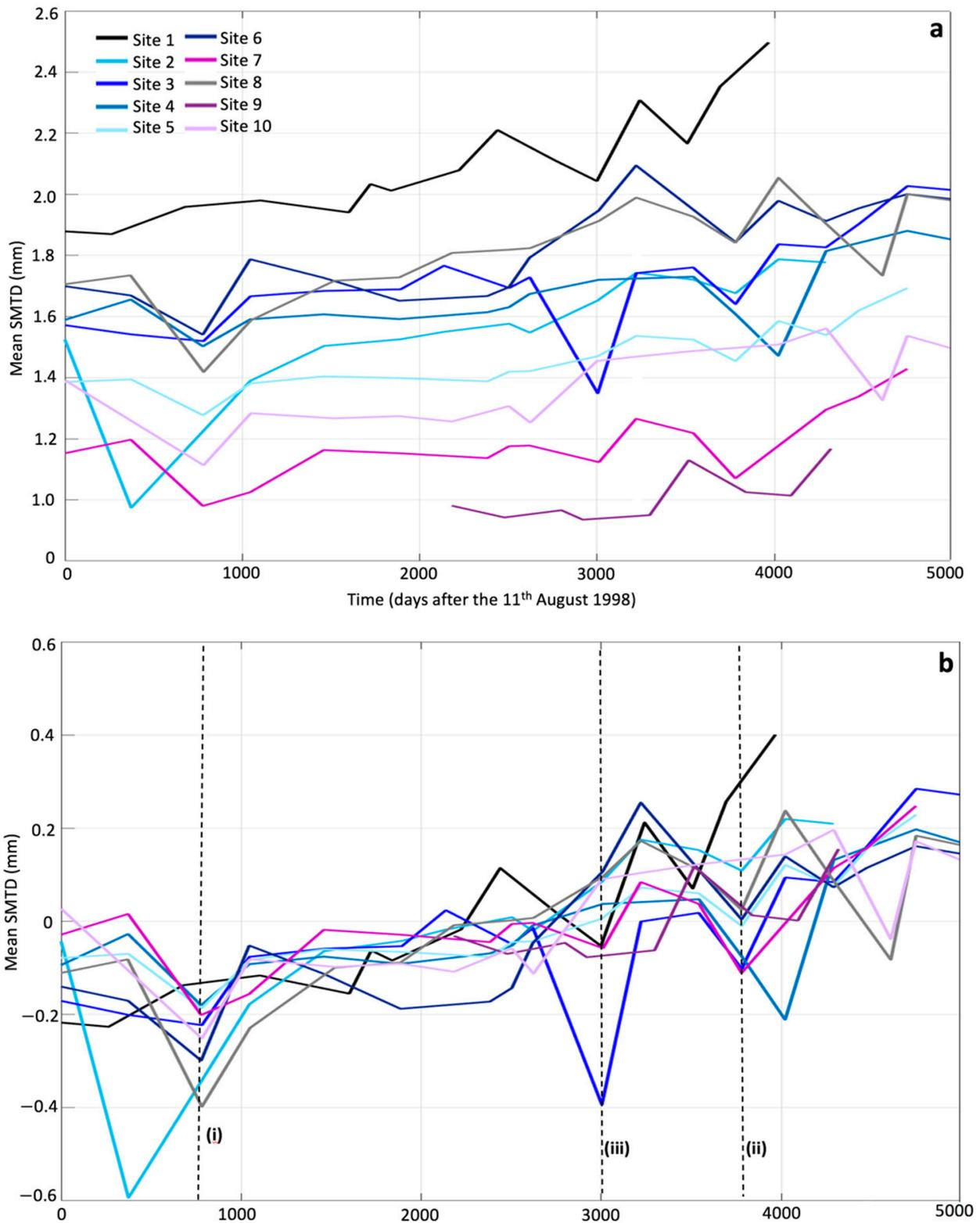
**Figure 2.** (a) Filtered mean sensor measured texture depth (SMTD) data for the northern sites on the A1. (b) Normalised mean SMTD data for the northern sites on the A1. (I) to (III) are “troughs” in data coinciding with severe rainfall events. (see text for further explanation).
