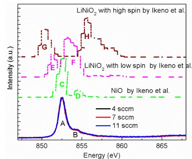
**Figure 4.** Ni  $L_3$  edge ELNES spectra of NiO thin films with different oxygen flow rates. The theoretical spectra of NiO and  $\text{LiNiO}_2$  calculated by Ikeno et al. [32] are presented for comparison. The intensity has been normalized by the height.
