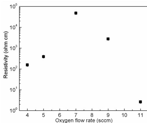
**Figure 3.** Room temperature resistivity of NiO thin films deposited on glass substrates with different oxygen flow rates.
