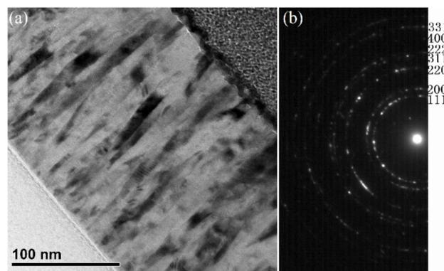
**Figure 2.** Bright field TEM image (a) and the electron diffraction pattern (b) of NiO thin films deposited with 11 sccm O<sub>2</sub> on Si (100) substrates.
