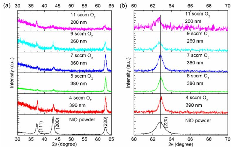
**Figure 1.** (a)  $\theta$ – $2\theta$  scan diffractograms of NiO thin films (200–390 nm) deposited on glass substrates with different oxygen flow rates. The deposition time was fixed at 6 min. The diffractogram of NiO powder is plotted at the bottom as a reference. (b) Magnified (220) diffraction peaks of NiO.
