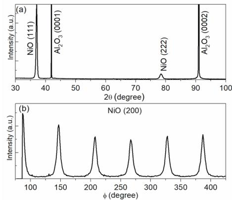
**Figure 5.** (a)  $\theta$ – $2\theta$  scan diffractograms of NiO thin films (about 200 nm thick) deposited on Al<sub>2</sub>O<sub>3</sub> (0001) substrates with 11 sccm oxygen flow; (b)  $\theta$ – $2\theta$  scan diffractogram of the (200) plane.
