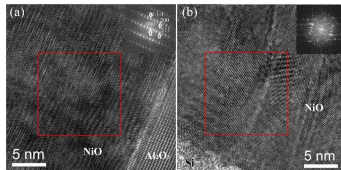
**Figure 6.** HRTEM images of an epitaxial NiO thin film on Al<sub>2</sub>O<sub>3</sub> substrate (a) and polycrystalline thin film on Si substrate (b). These films were deposited at the same time. Insets show the FFT patterns of selected regions marked by red frames.
