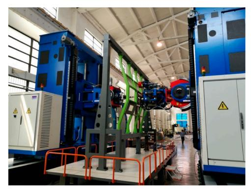
Figure 8. Automatic drilling and riveting machine pressure riveting test.
