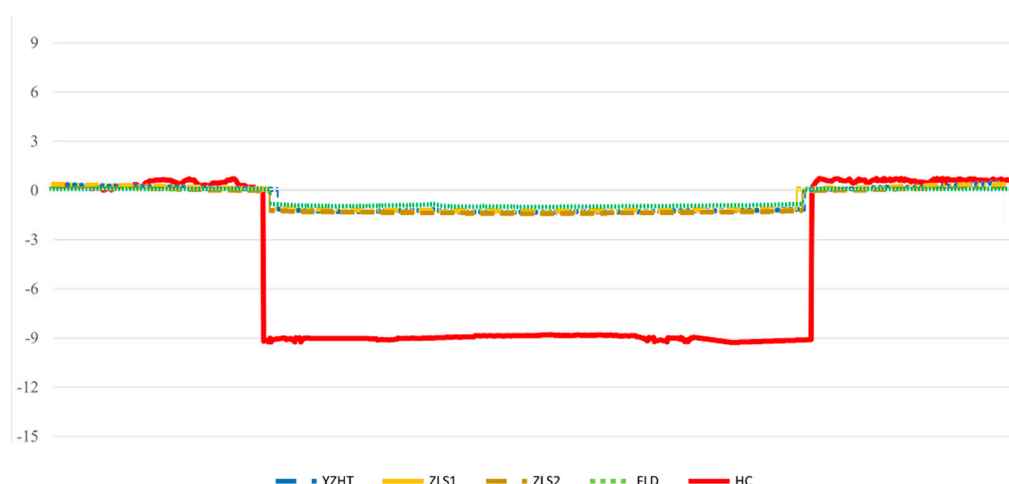
Figure 6. Surface profiles of representative specimens from according to the ceramic material (YZHT, FDL, ZLS1, ZLS2 and HC) after 15 years of toothbrushing simulation.
