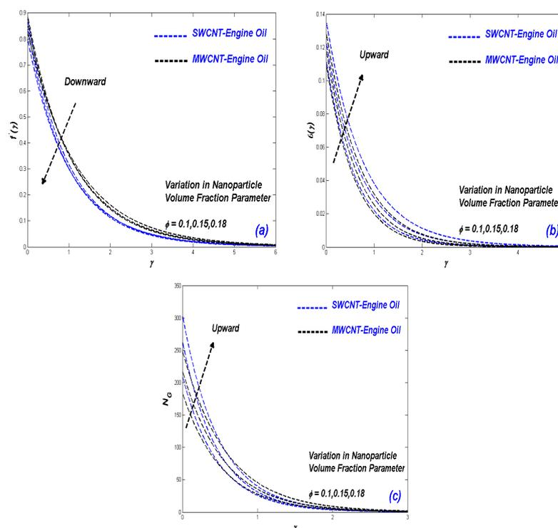
Figure 8. (a) Velocity change with  $\phi$ ; (b) Temperature change with  $\phi$ ; (c) Entropy change with  $\phi$ .
