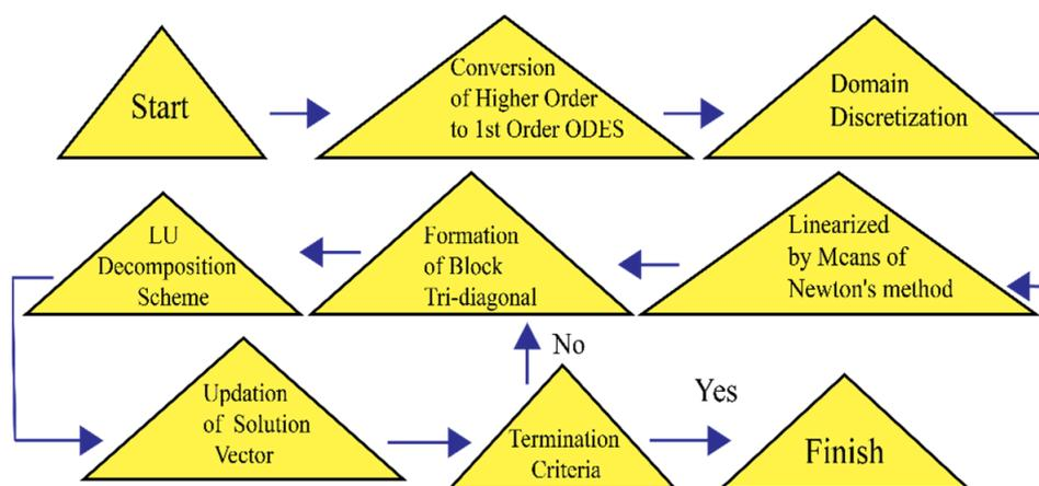
Figure 4. Flow chart of Keller-box method.
