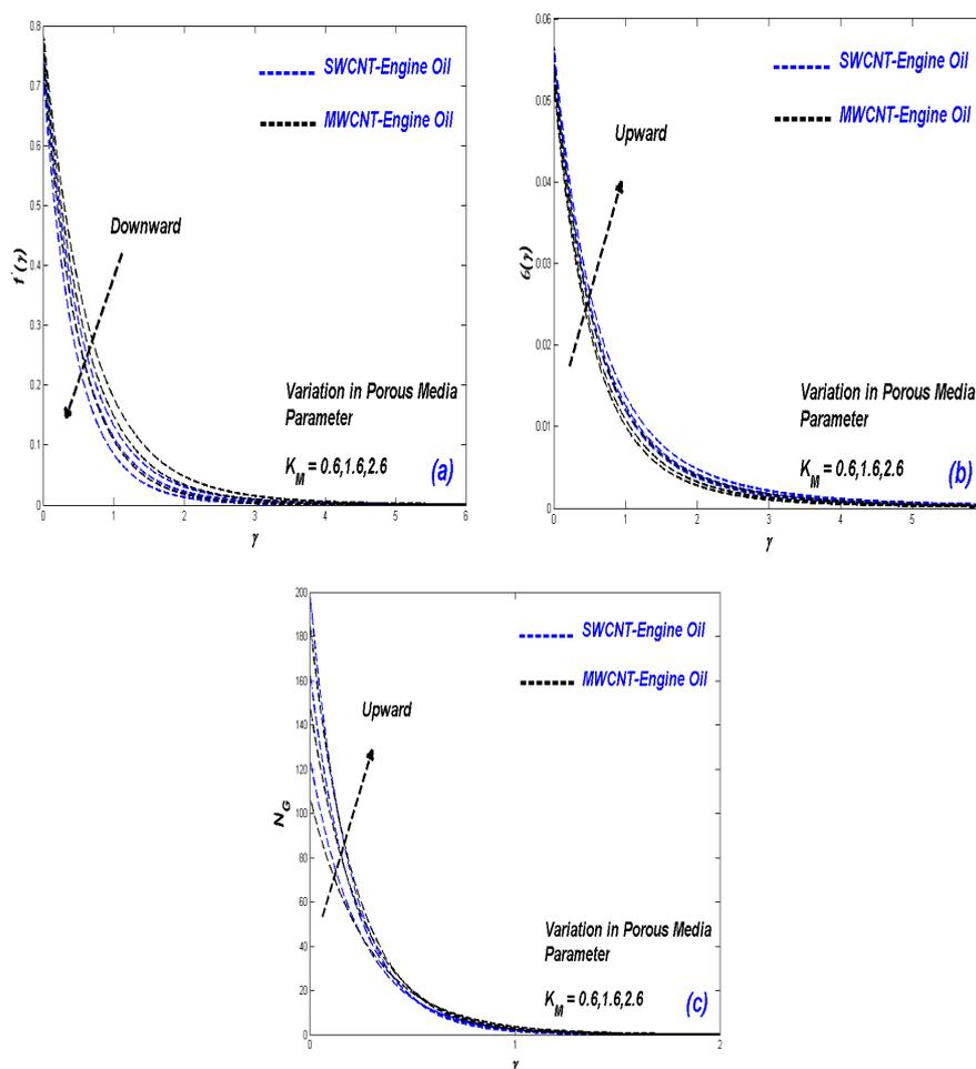
Figure 6. (a) Velocity change with  $k_M$ ; (b) Temperature change with  $k_M$ ; (c) Entropy change with  $k_M$ .
