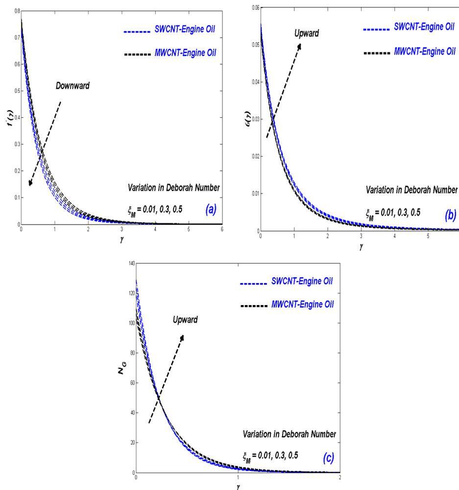
Figure 5. (a) Velocity change with  $\zeta_M$ ; (b) Temperature change with  $\zeta_M$ ; (c) Entropy change with  $\zeta_M$ .
