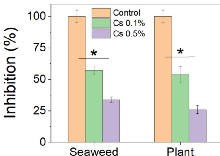
**Figure 9.** Antimicrobial effect of chitosan-coated paper was assessed by measuring the degree of inhibition (%) of *E. coli* growth on seaweed (High S%) paper and plant paper coated with chitosan (M-Cs) (\*  $p < 0.05$ ).
