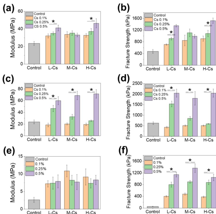
**Figure 8.** Tensile moduli and fracture strength of (a,b) Low S% seaweed paper, (c,d) High S% seaweed paper and (e,f) plant paper coated with chitosan with varying concentrations and molecular weights  $M_W$  (\*  $p < 0.05$ ). Uncoated papers were used as control.
