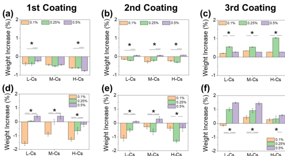
**Figure 4.** The increase in weight of paper samples after dip coating with chitosan: (a–c) Low S% seaweed paper and (d–f) High S% seaweed paper. The coating was performed up to three iterations (\*  $p < 0.05$ ).
