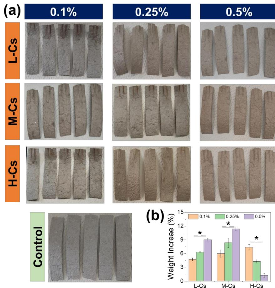
**Figure 5.** (a) Photographs of plant papers coated with chitosan with varying concentrations and molecular weights. (b) The increase in weight of plant papers after chitosan coating (\*  $p < 0.05$ ).
