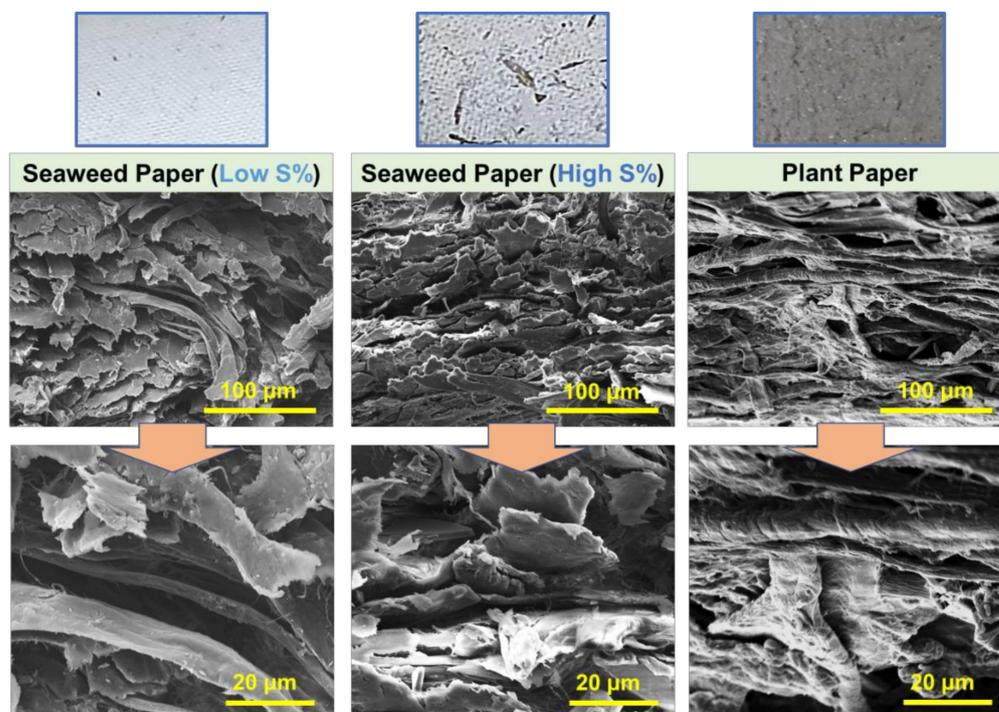
**Figure 3.** Photographs and SEM images of seaweed papers with different seaweed pulp contents (Low and High S%) and plant paper.
