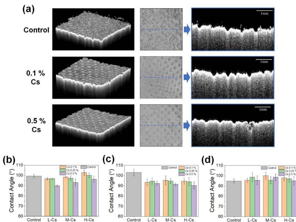
**Figure 10.** (a) OCT imaging of the surface of seaweed paper (High S%) coated with varying chitosan concentrations; 0% (control), 0.1% and 0.5%. Three-dimensional and cross-sectional (along the dotted line) views are presented. Water contact angles measured on chitosan-coated papers: (b) Low S% seaweed paper, (c) High S% seaweed paper and (d) plant paper. Uncoated papers were used as control.
