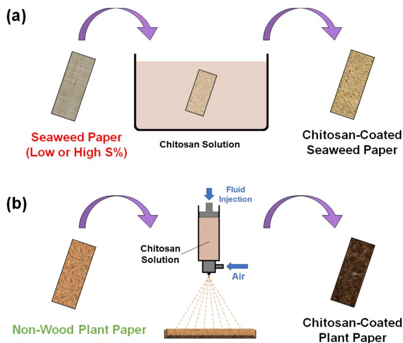
Figure 1. Chitosan was coated on (a) seaweed paper by dip coating or (b) plant paper by spray coating.
