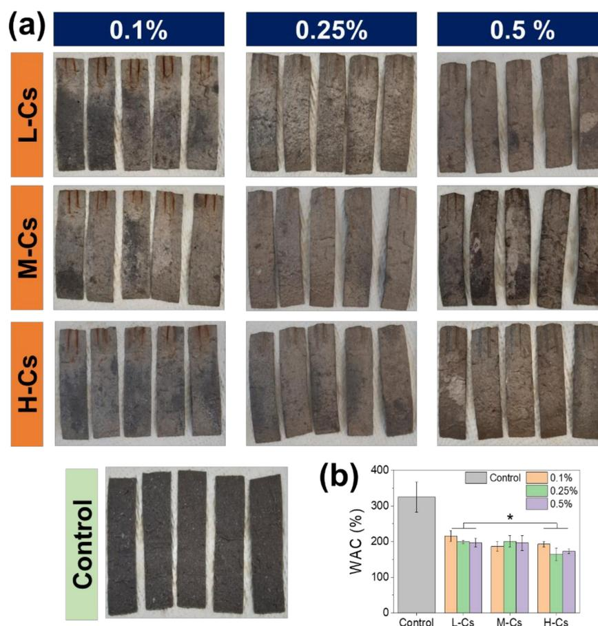
**Figure 7.** (a) Photographs of plant paper samples coated with chitosan with varying concentrations and molecular weights after immersing them in hot water. (b) Water absorption capacity (WAC) values of plant papers coated with chitosan (\*  $p < 0.05$ ). Uncoated paper was used as control.
