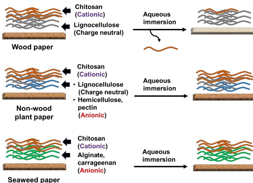
Figure 2. Schematic illustration of wood, non-wood plant and seaweed papers coated with chitosan with different binding affinities. Non-wood plant and seaweed papers having anionic components demonstrate higher binding affinities than wood paper, which is charge neutral.
