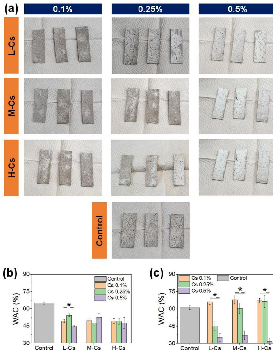
**Figure 6.** (a) Photographs of seaweed paper samples (High S%) coated with chitosan with varying concentrations and molecular weights, after immersing them in hot water. Water absorption capacity (WAC) values of (b) High S% and (c) Low S% seaweed papers coated with chitosan (\*  $p < 0.05$ ). Uncoated papers were used as control.
