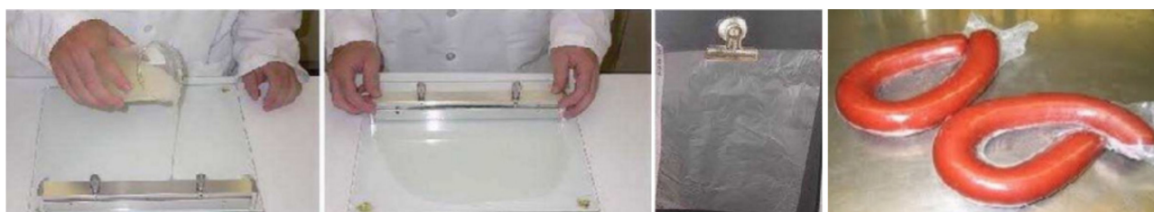
Figure 1. A simple lab process for making edible films from gum and examples of the sausage packaging. Reprinted from [15,16]. Copyright 2009 Springer.
