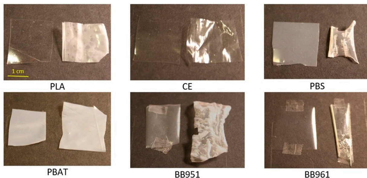
Figure 1. Pictures of the bioplastics before (left) and after (right) exposure to MilliQ water for 3 h at 80 °C. The treatment modifies the transparency properties of the polymers, sometimes in a severe way. In the best cases (CE and PBAT), only some wrinkling is observable. For bilayer materials, a mismatch in the shrinking of the polymer sheets is also observed.
