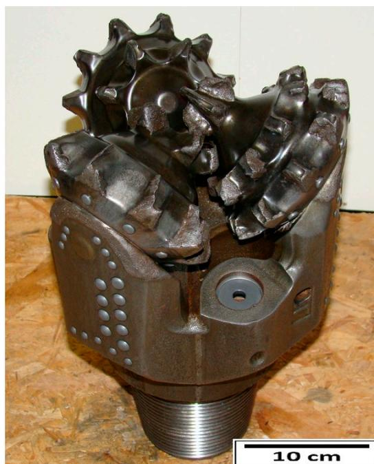
**Figure 4.** Worn roller cone drill bit ( $\varnothing$ 215.9 mm) after drilled interval.
