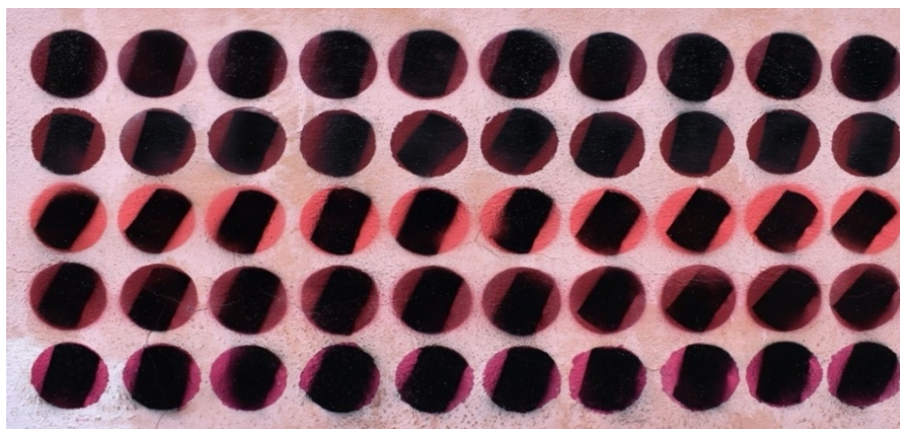
Figure 1. Vandalism carried out on selected specimens for cleaning tests.
