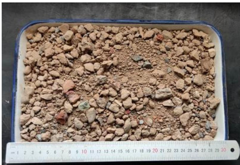
**Figure 1.** Recycled aggregates from C&D materials.
