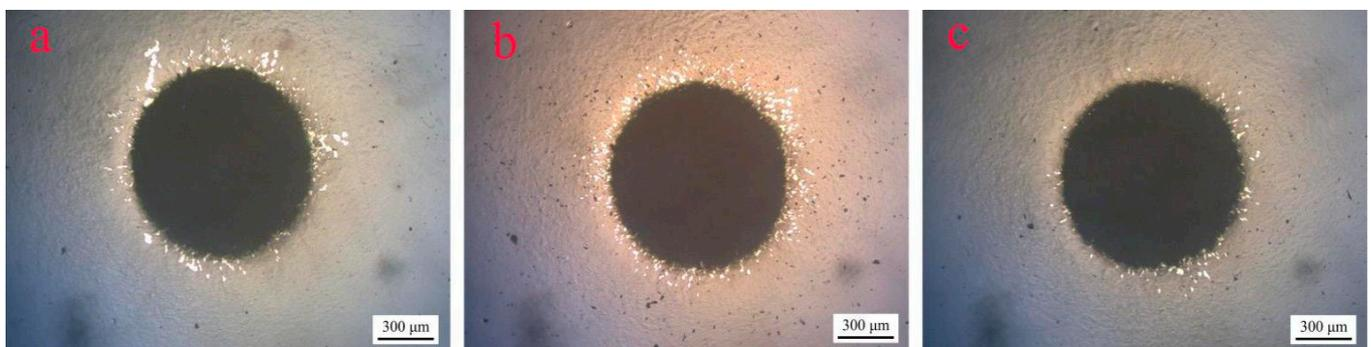
**Figure 11.** Optical micrograph of  $\text{MoS}_2\text{-Ti}_L/\text{MoS}_2\text{-Ti}_H$  coatings after Rockwell-C indentation: (a) sample S300-900; (b) sample S600-600; (c) sample S900-300.
