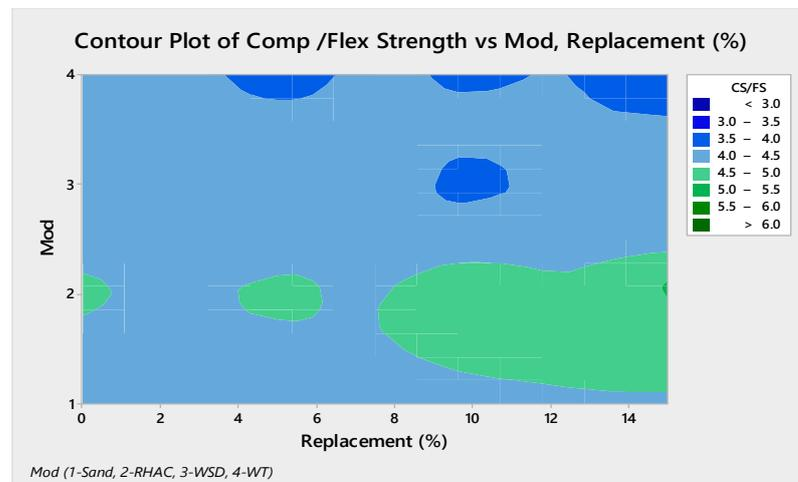
Figure 7. Contour plot of compressive/flexural strength (MPa) vs. mod, replacement (%).
