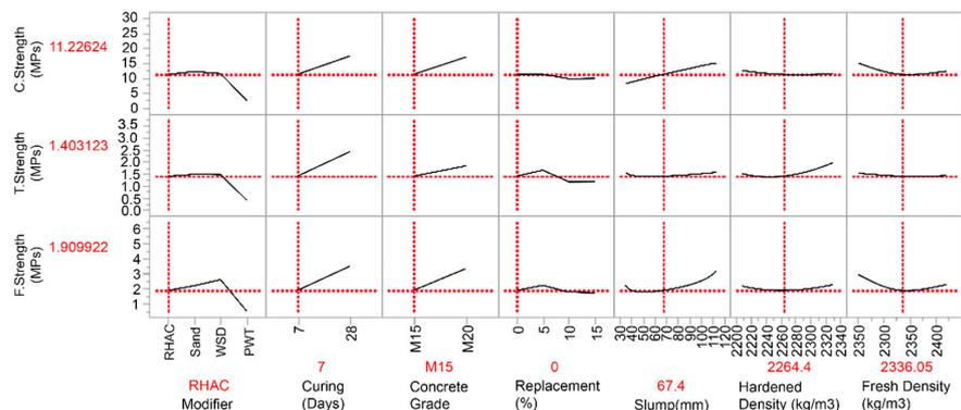
Figure 6. Prediction profile graph for the analysis of mechanical properties of green concrete.
