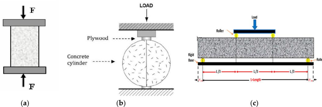
**Figure 3.** Strength testing machine mechanism (a) compressive, (b) tensile, (c) flexural tests.
