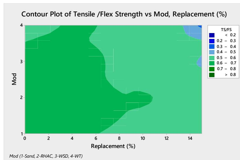
**Figure 8.** Contour plot of tensile/flexural strength (MPa) vs. mod, replacement (%).
