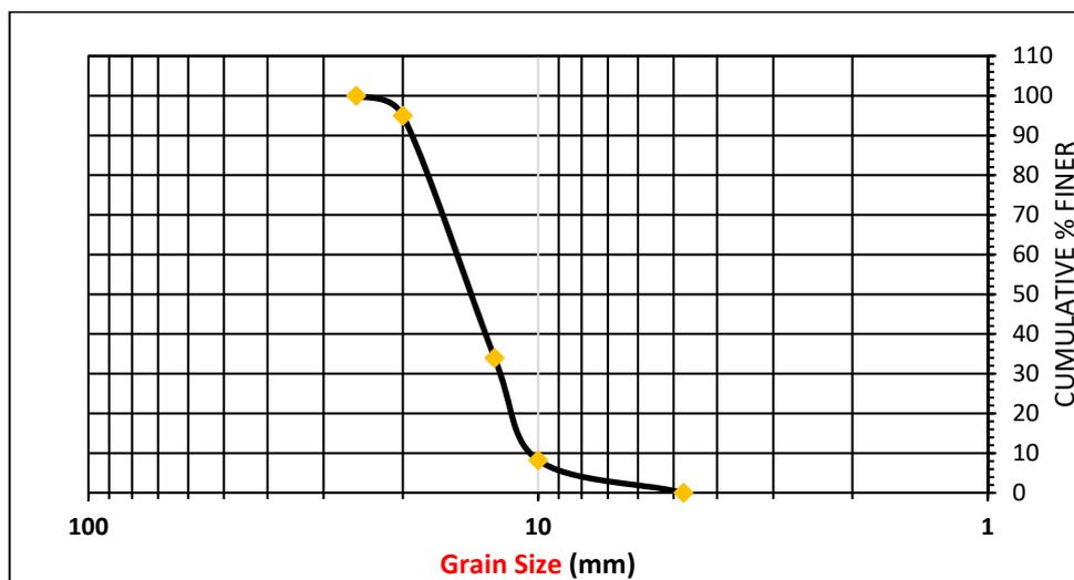
Figure 2. Coarse aggregate sieve analysis.
