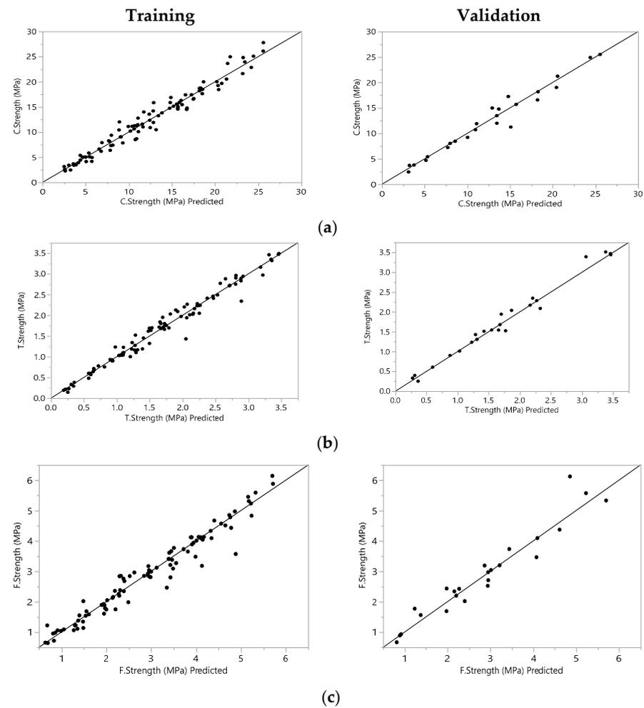
**Figure 9.** Training and validation plots for (a) compressiv strength, (b) tensile strength, (c) flexu-ral strength.
