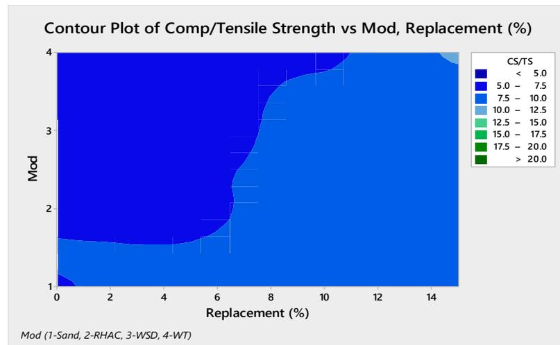
Figure 5. Contour plot of compressive/tensile strength (MPa) vs. mod, replacement (%).
