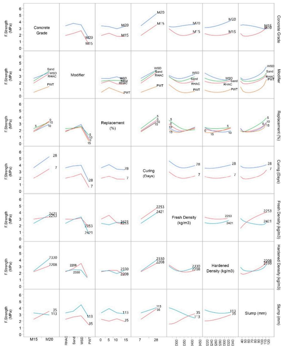
Figure 12. Flexure strength interaction profile.
